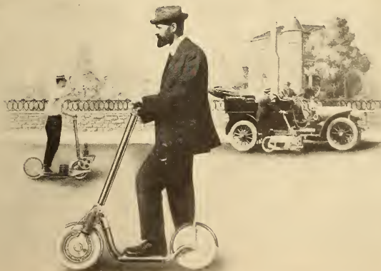
Hugo C. Gibson, the well known automobile engineer, has brought out a novel two wheeled vehicle called the "Autoped," resembling a huge roller skate. It is driven by a small gasoline engine, and the whole device weighs 40 pounds.
