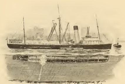
Showing How the Steel Shaft Plunged Through the Bottom of the Ship
