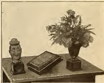
VARIOUS FORMS ADAPTED TO THE TRANSMITTER AND RECEIVER OF A HOUSEHOLD LOUD SPEAKING TELEPHONE
