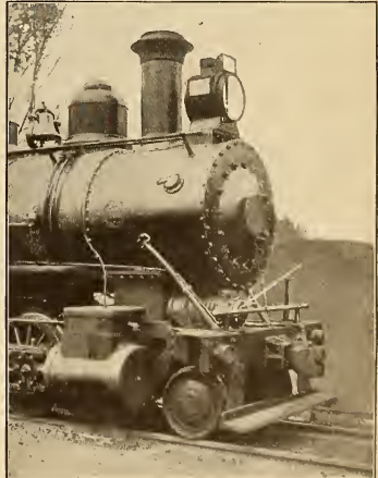
THE ARROW SHOWS THE LOCATION OF THE LIGHTING GENERATOR ON THE LOCOMOTIVE
