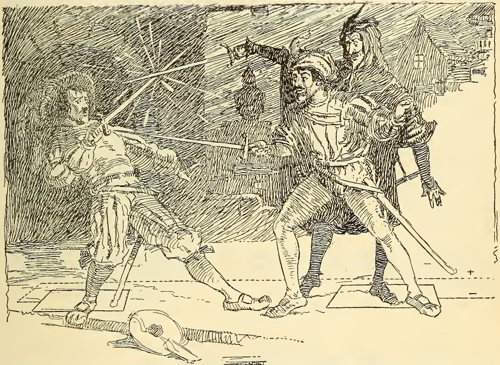
FIG. 8. IN WHICH THE CONTACT PLATE METHOD IS USED, CURRENT BEING CONDUCTED TO THE SWORDS THROUGH CONCEALED WIRES IN THE CLOTHING
