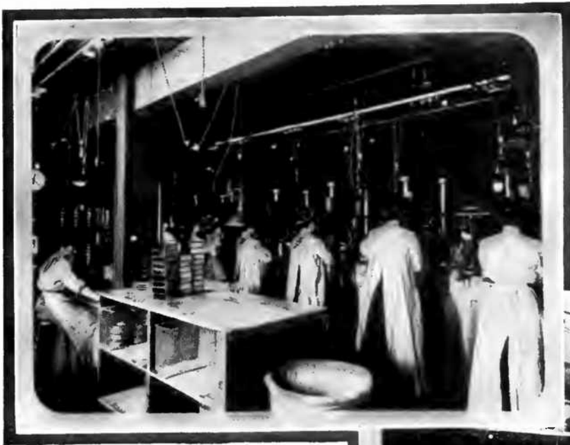
A Battery of Projecting Machines Operated by Women Who Inspect Finished Film Before It is Allowed to Leave the Factory. Imperfect Film Is Destroyed.
