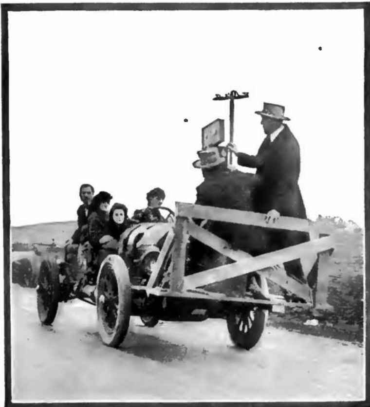
Wooden Platform Fastened to a Racing Automobile, in Order to Hold the Camera, Operator and Director.
