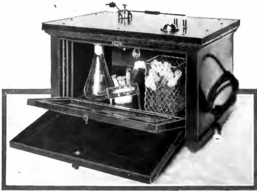
An Electrically Heated Incubator for the Culture of Bacilli. The Heat Is Automatically Maintained at Any Desired Temperature.
