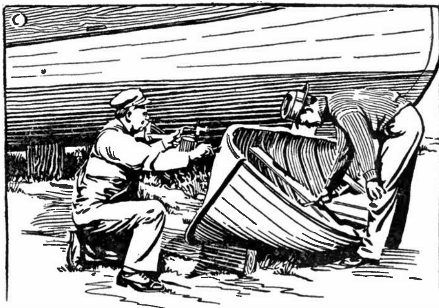
If the Varnish on a Boat is in Poor Condition, It is Better to Remove It Entirely and Then Refinish.
