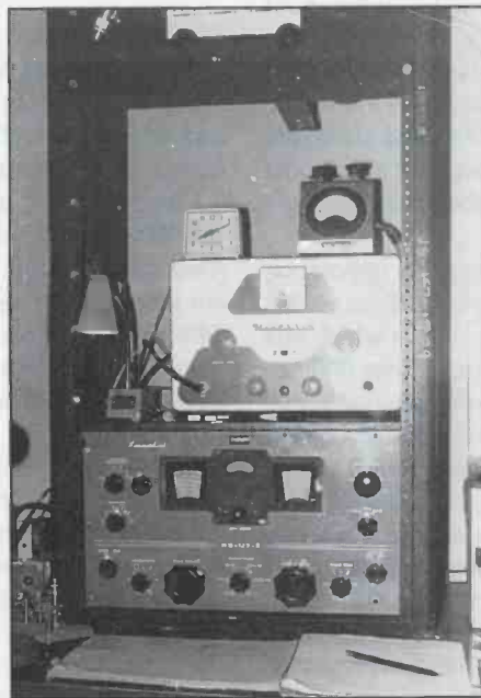
Robert's station photo from '71 with home-brew SWR bridge, Hammarlund HQ-129X receiver, and Heath DX-40 transmitter. The QSL at top of the photo is made from an 80-column IBM punch card.
