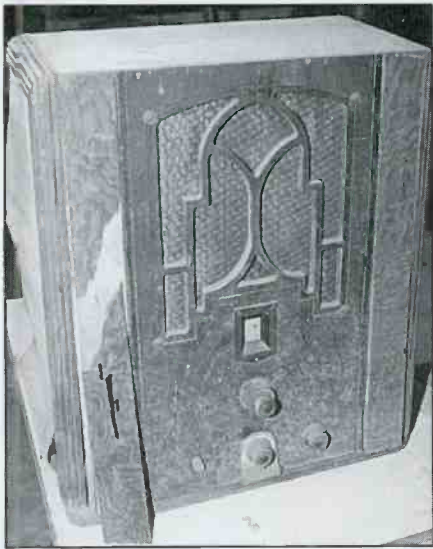
Front of the American Bosch tombstone. Notice how the oak burl veneer has lifted, and broken away from the front panel. Notice the warped side panel.
