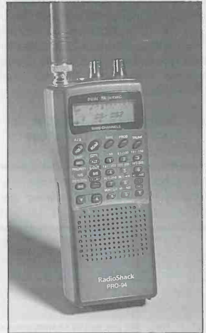
RadioShack's new PRO-94 handheld scanner has 20 priority channels and service search with preset frequencies.
