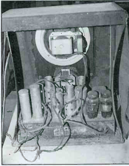
The rear view tells all. The sides are completely destroyed from decades of moisture. The chassis is coated with dirt, and the chassis side aprons are rusted through.
