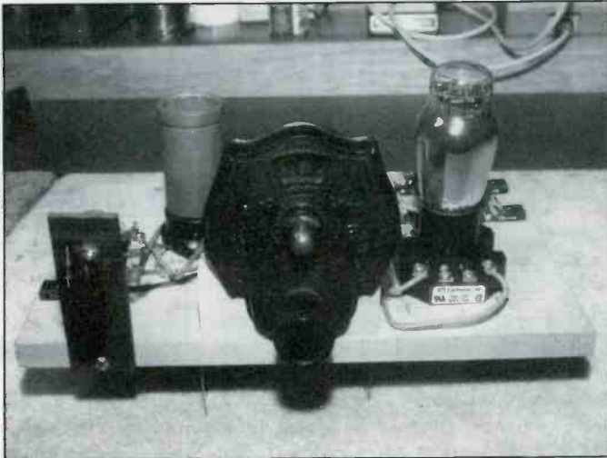
Rear view of the receiver makes a good guide for parts placement.
