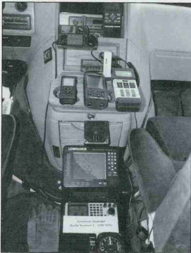
Birdies from the engine computer were so strong that low-band scanning was impossible. The problem was solved by shielding the fiberglass engine cover.
