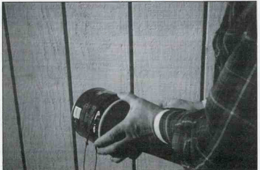
Wrapping the coax around our coffee can to make a balun.
