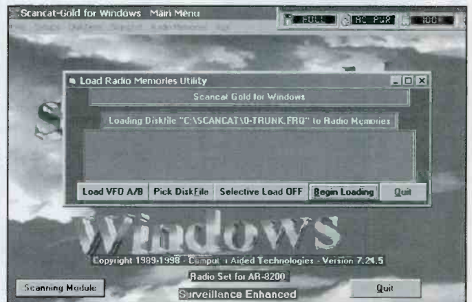
Here's the screen used to download frequencies to your radio's memories, if that function is supported.
