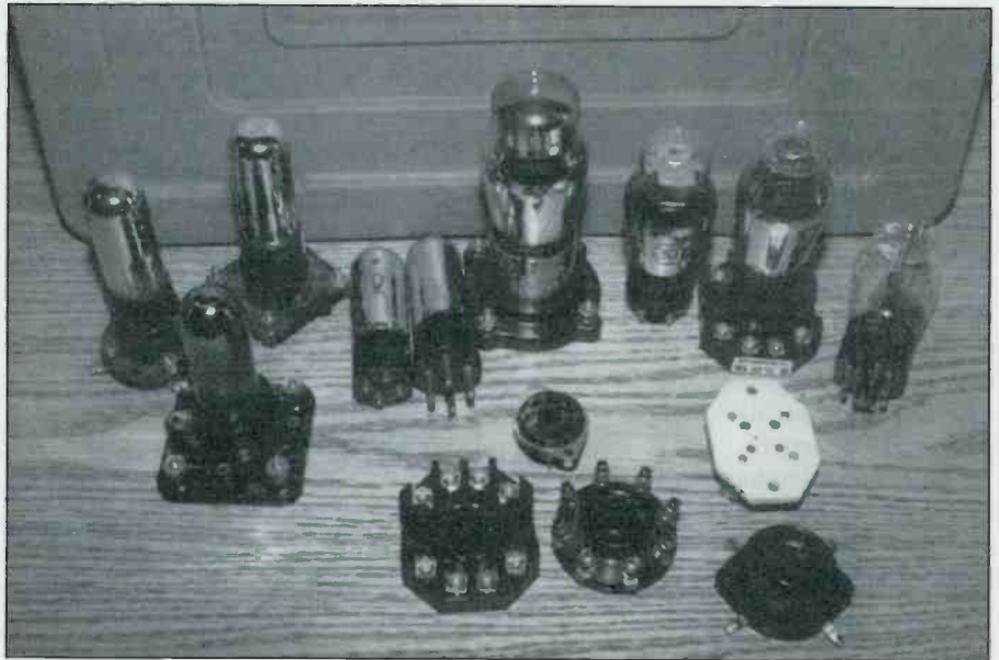
The three tubular tubes at far left are '99 types in sockets. The taller standing pair in the rear is UX based, the shorter '99 is a UV base. Note the difference between the UX and UV pin style by comparing the two '99 tubes laying on their side. Front and center is a UX201, with a metal twist-lock base. Continuing to the right is a type '30, a 1H4 in an octal relay socket, and last, a 1H4 laying on its side. The three octal sockets are shown in the center, a modern relay socket, a chassis mount, and a vintage breadboard mount. Two four-pin sockets are shown at far right. Tubes at left are "tubular" shape, tubes at right are "ST" shape.
