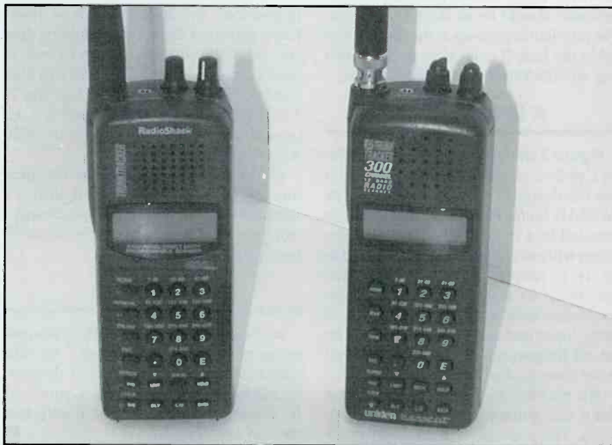
These almost-twin handhelds changed the world of scanning. For the first time, it became possible to follow the popular Motorola Type II trunking used by so many public safety agencies. Shown are the RadioShack PRO-90 and the Uniden BC-235. They are functionally identical.
