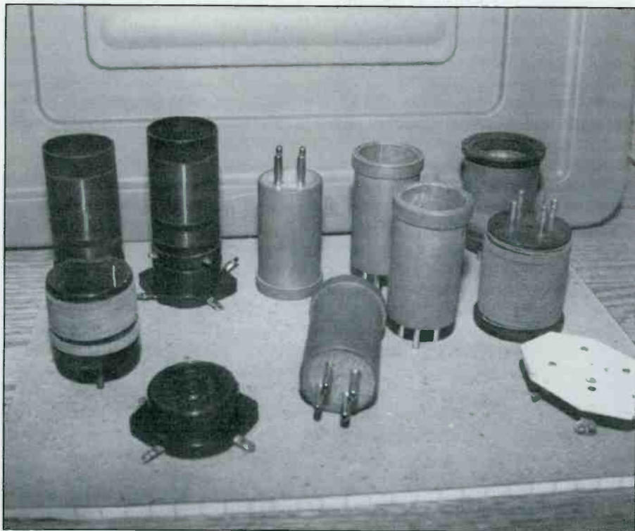
Plug-coil forms. At left are some examples of commercially-made and homebrew coil forms. The four 4-pin forms in the center were purchased from Ocean State Electronics. At far right are two examples of 5-pin forms. Front left shows a flush mounting 4-pin breadboard socket. The socket at far right is made from low-loss Isolantite material.
