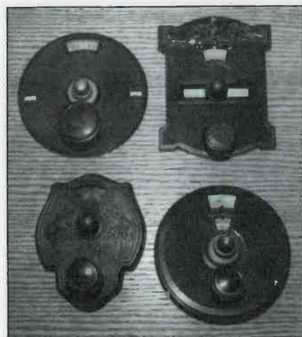
1920s-style vintage dial verniers. Note that all styles have 0-100 logging scales; two styles also offer "write-in" areas to pencil in station call letters.
