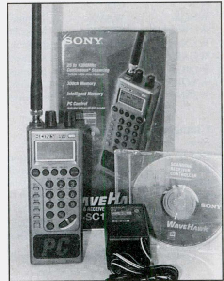
The Sony SC1PC is a full-featured scanner with a complete computer interface. The radio features 300 channels in 10 "pages" of 30 memories each.
