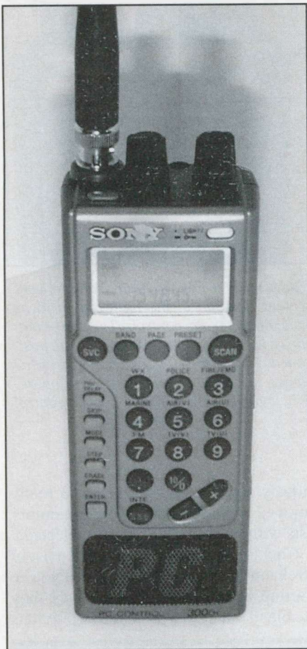
The SC1PC runs on "AA" batteries or off the included wall power supply. The PC version also comes with software for receiver control and a database of frequencies (Spectrum by Percon) on the CD ROM.
