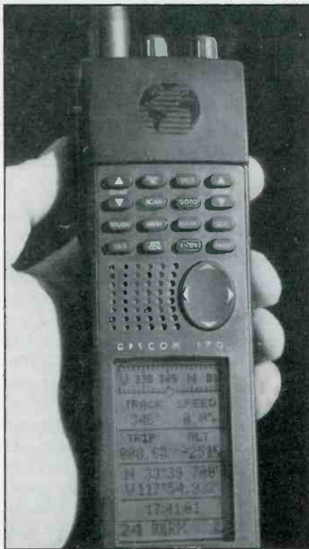
This combination radio/GPS receiver can run on NiMH cells, giving you extended running time.
