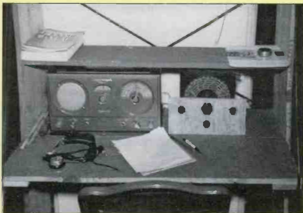
W9JTN's first SWL set-up in 1948 NC-33, RME preselector, long wire
