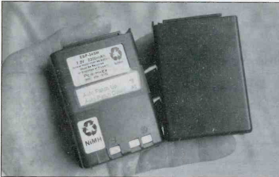
They're the same size, but the battery on the left has almost twice the capacity as the nickel cadmium (NiCd) on the right.
