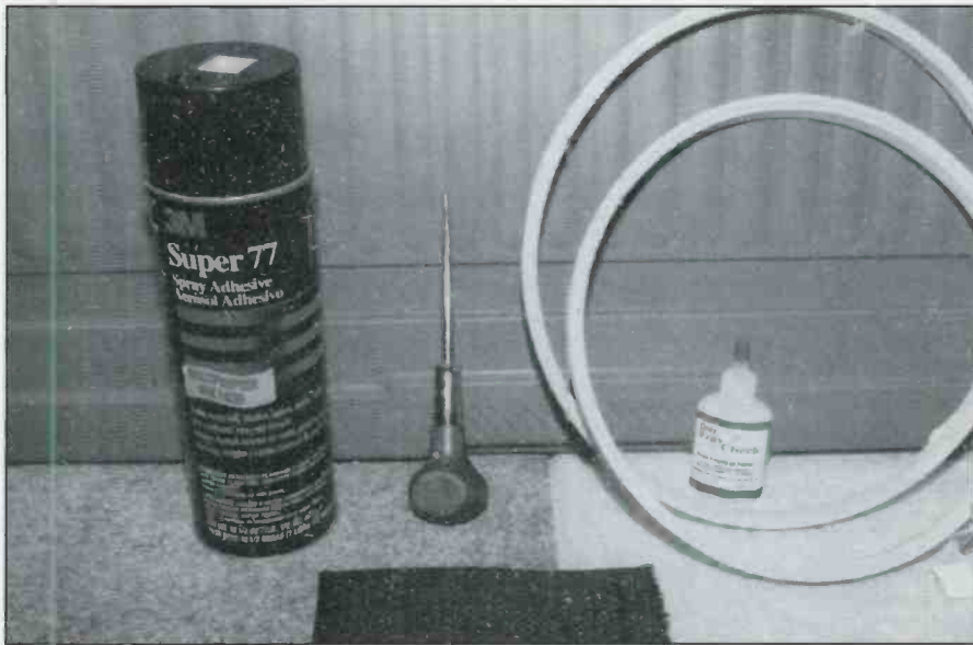
Here are the tools of the trade. A spray can of 3M Super 77 spray adhesive, a sharp pointed awl, embroidery hoops, Spritz Fray Check, and the new grille material are what we need to get started.
