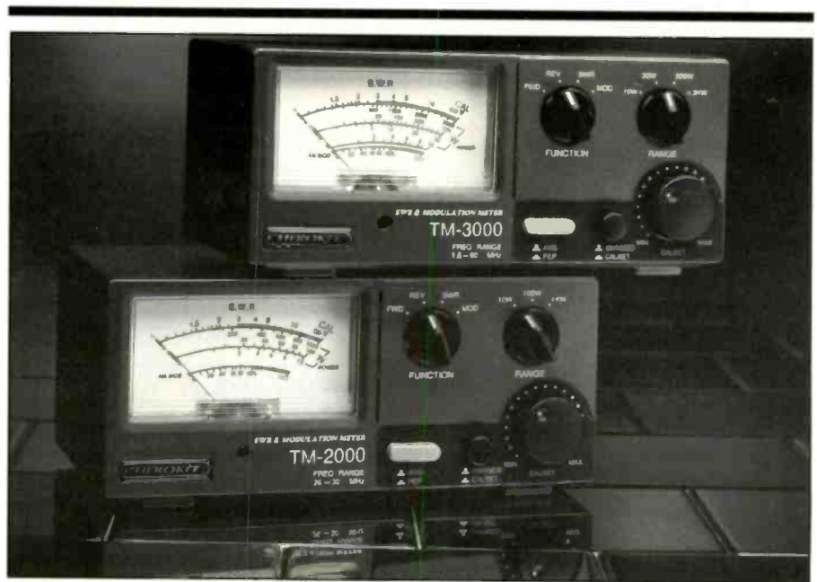
Cherokee's TM-2000 and TM-3000 SWR/power/modulation meters work as good as they look.
