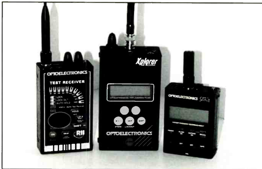
Frequency counters and "near field" devices can help you search for new frequencies or look for frequencies in use at a scene or event. Shown are the R-11 (no counter, but audio), the top-of-the-line Xplorer (audio and counter functions), and the Scout (no audio, but can interact directly with some scanners); all from Optoelectronics.
