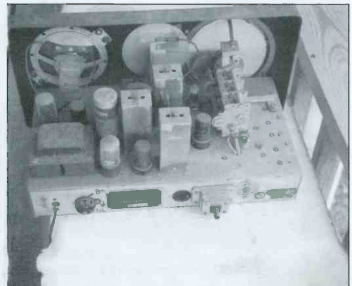
Rusty tubes, dirt, and grime — certainly a sad condition for a once-proud receiver like the S-40A.
