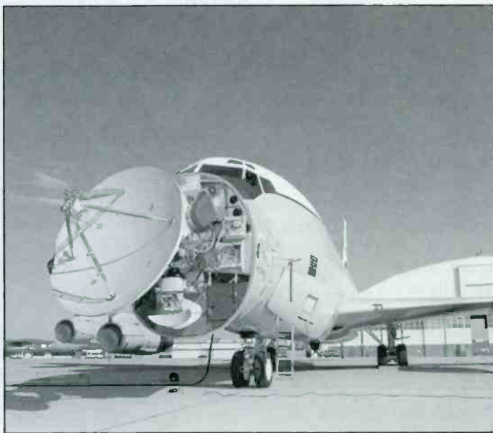
The drooped nose of the EC-18 contains a steerable radar dish. (USAF Photo) ↓
