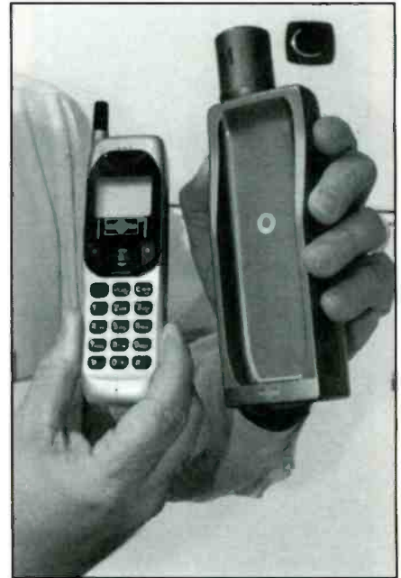
The hi-tech "docking booster" (on right) turns the Iridium Motorola cellular phone into a satellite phone.
