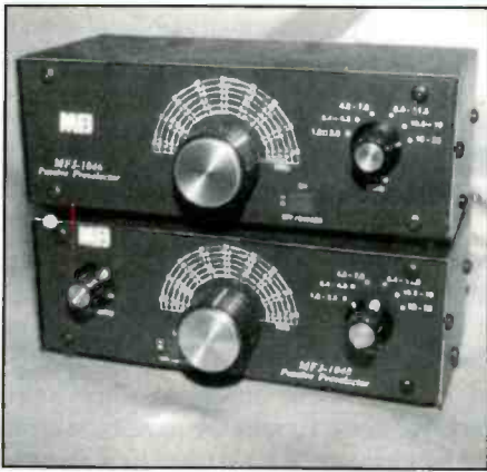
The MFJ-1046 and MFJ-1048 preselectors. Either unit is ideal for use with an SWL receiver, but the MFJ-1048 also incorporates RF sensing for automatic by-passing when used with a transceiver.
