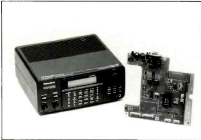
A peek at the pipes behind the wall. The OS board installs inside your radio.
