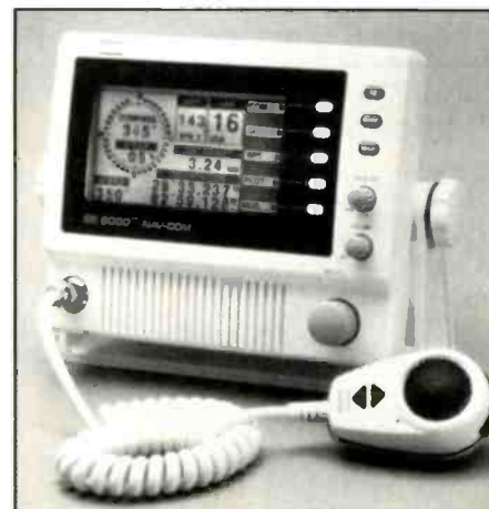
This Nav-Com marine VHF set will also transmit your GPS position as a packet on 156.525 MHz.
