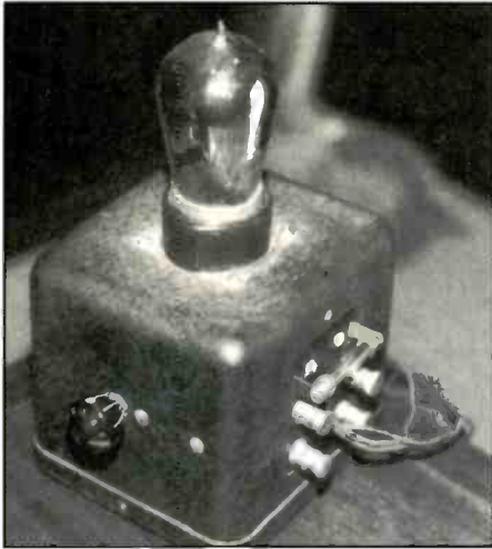
Crosley one-tube "Pup" with an early '01A style tipped-brass base tube. Many of the Crosley battery sets were housed in plain and spartan enclosures.
