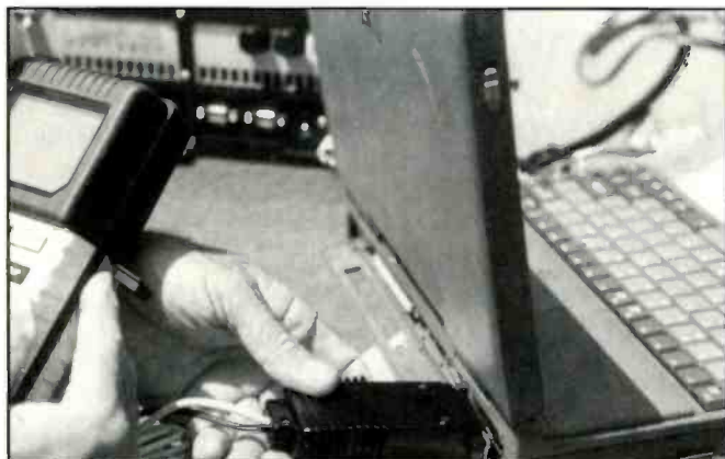
Hooking up a GPS to the laptop and a ham A.P.R.S. unit will squawk your position worldwide.
