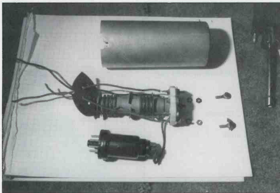
Inside view of a typical vintage IF transformer. Upper ceramic plate has two compression mica trimmer capacitors for alignment. Note the flying grid lead going to the IF stage tube. When replacing leads great care must be taken not to damage the fine wires used on the coil windings.
