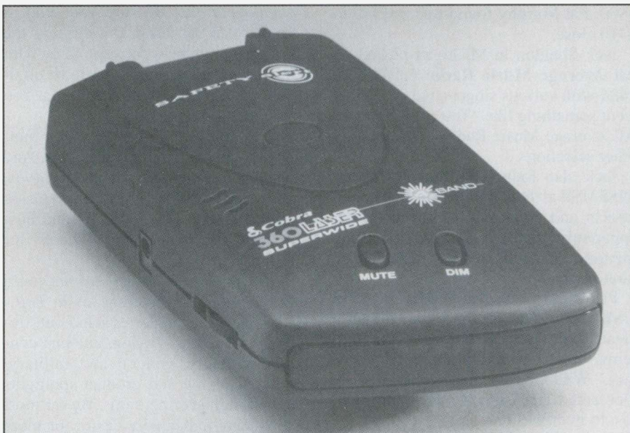
The Cobra "Trapshooter" is a super-wideband radar/laser detector and also receives the new SWS messages. (Courtesy Cobra Electronics Corp.)
