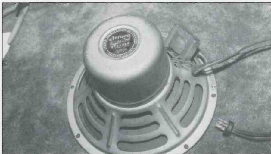
This electrodynamic speaker is from an American Bosch console. Note the shield covering the massive field coil winding. The audio stage output transformer is mounted on the speaker frame. These speakers aren't hi-fi, but were well matched to the program material of the day. The wire leads on this speaker assembly carry dangerous voltages! If the wires show any sign of age such as cracking insulation, they must be replaced.
