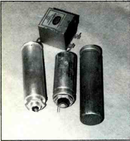
Photo B: Typical vintage electrolytic capacitors, circa 1930s, usually rated at 8 mFd and 450 volts. The round metal can styles either had a large mounting nut for attaching to the chassis, or were held in place with special clamping hardware. One example has an isolated can, the negative and positive leads were brought out with cloth-covered wires. The other style used a large solder lug for making the positive connection.
