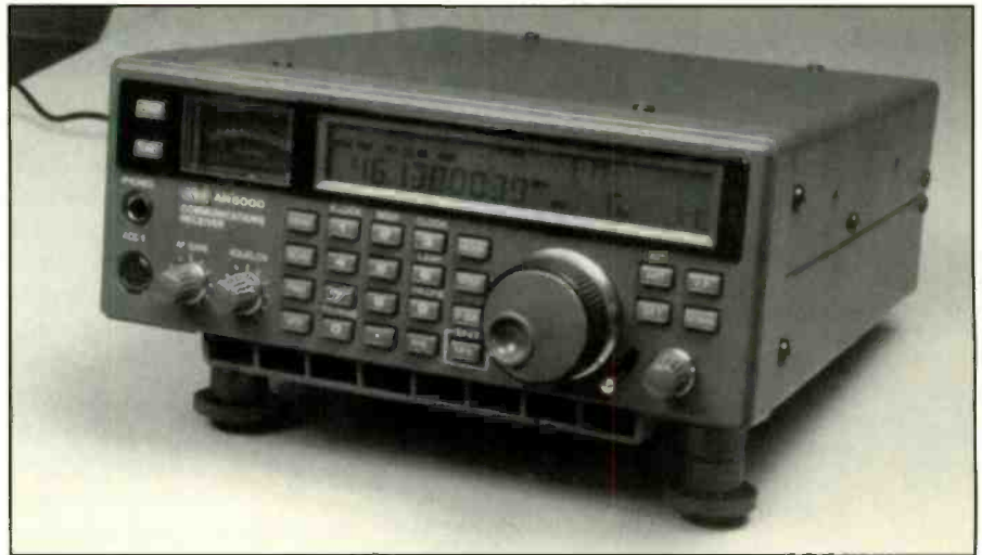
The AR5000 is a high-performance wideband all-mode receiver that covers 10 kHz to 2600 MHz. Housed in a metal cabinet, it is powered by an external 12 Vdc power unit, but may be operated from any regulated supply or battery capable of providing 12 to 16 Vdc at 1 amp. (Courtesy AOR).
