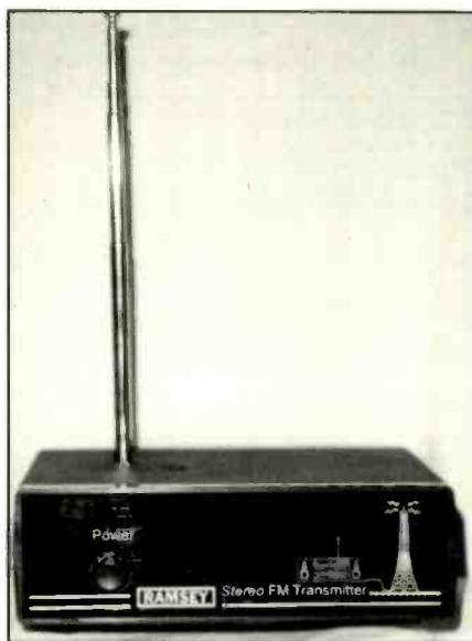
A look at the Ramsey Stereo FM Transmitter. Assembly is easy and straightforward. You'll have plenty of fun building and using these transmitters.
