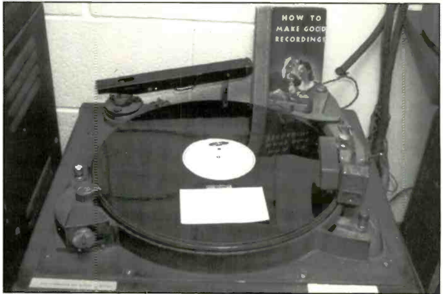
WMPC's record lathe once used for cutting electrical transcription discs.
