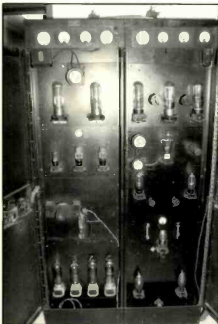
From 1935 to 1967, WMPC used this Doolittle and Faulkner 250 watt transmitter. The station has it on display.
