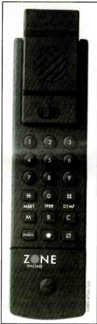
Shown above is England's Zonephone, an 800-MHz digital communications service offered as a low-cost alternative to cellphones.
