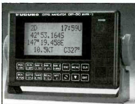
GPS readouts can spot a distress call position within a 300-foot circle 95 percent of the time.
