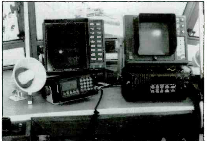
Lifeguard rescue boat bridge station electronics are all rated splash-proof.
