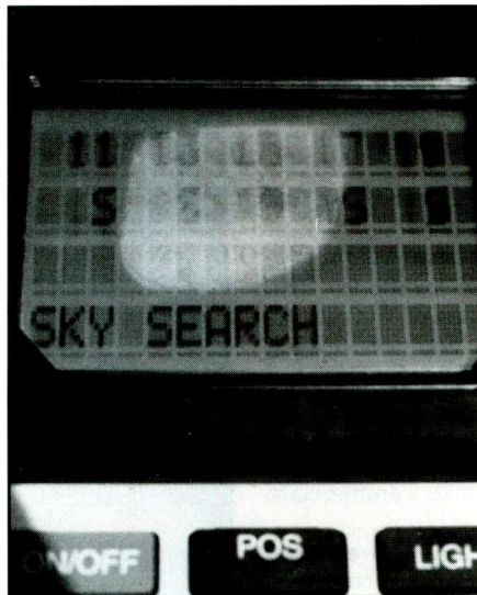
Moisture encased in the display window indicates wet "insides" (or parts) that need to be dried out.
