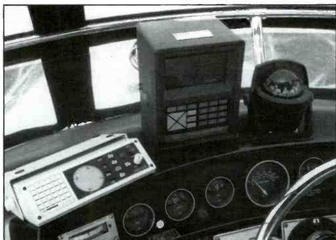
Combination VHF radio and automatic direction finder.
