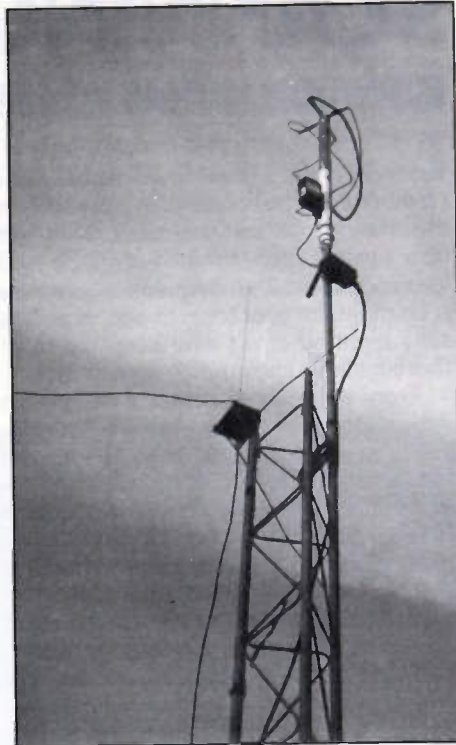
The Quadrifilar helix antenna shown above is considered most unusual.
