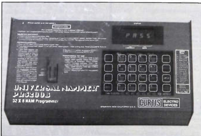
The PR-5200B can program a NAM into most cellphone models in about a minute.
