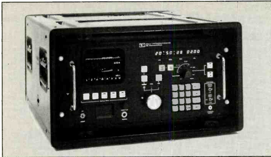
Figure 3. An ionosonde receiver. Photo courtesy Gerald Oicles/BR Communications, Sunnyvale, CA
