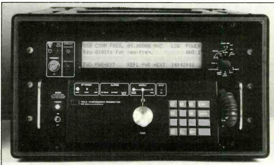
Figure 2. An ionosonde transmitter. Photo courtesy Gerald Oicles/BR Communications, Sunnyvale, CA
