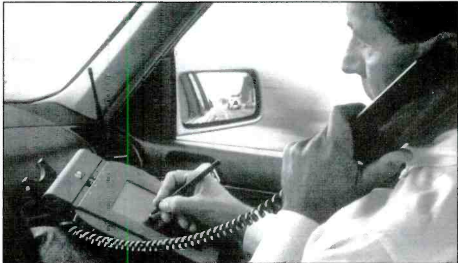
The EO Personal Communicator 440 shown in use with optional cellular phone module. It allows E-mail, FAX, PC, and all sorts of modes from the field. Lets you communicate anytime, anyway, anywhere. An interesting concept.
