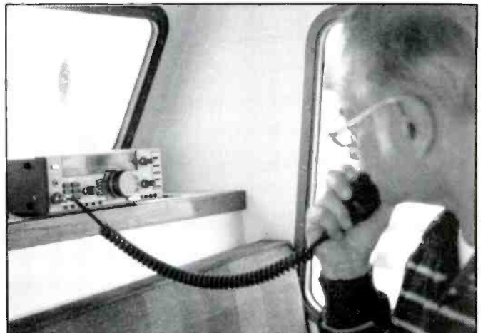
Most SSB and commercial marine mikes use a noise cancelling element, and must be held close to your mouth for full power output.
