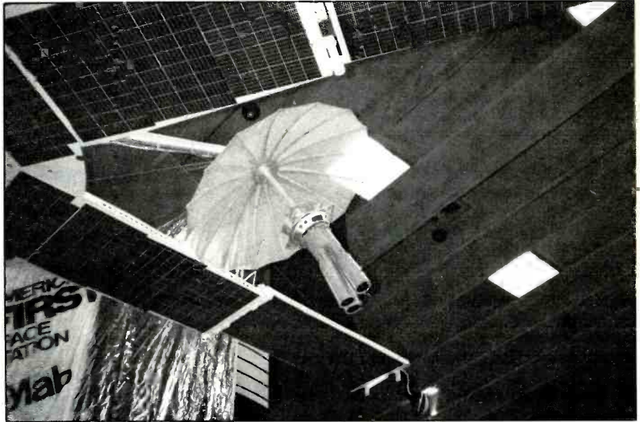
The Molniya carries two dish/horn antenna combinations that operate at 800 MHz and 1 GHz.
