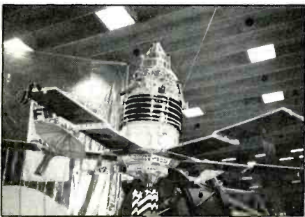
The Molniya 1 satellite is a military comsat that uses a highly elliptical orbit.
