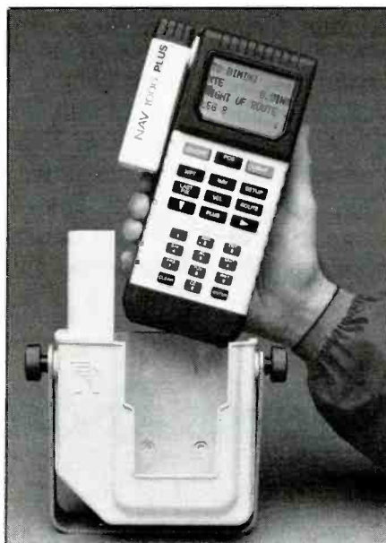
For fixed use, the portable GPS slides into the mounting bracket.
