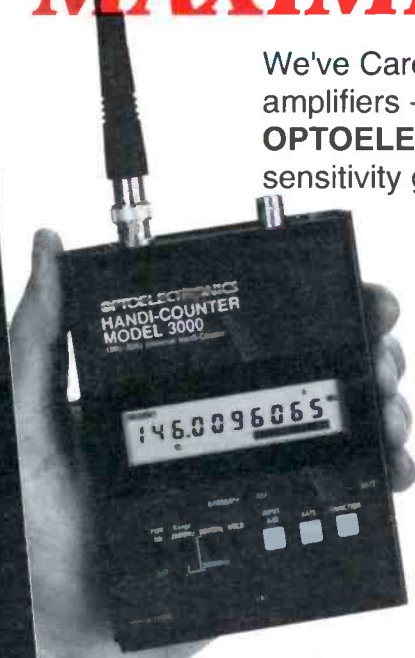
MODEL 3000 Multi-function Counter 10Hz-3GHz, 10 Digit LCD with frequency, period, ratio, interval & signal level bargraph...$375.
