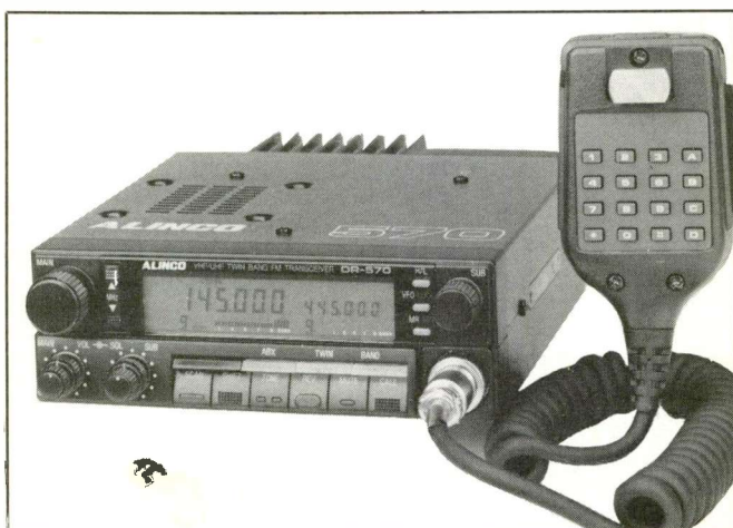
Alinco DR-570 tunes in 800 MHz with a simple modification.
