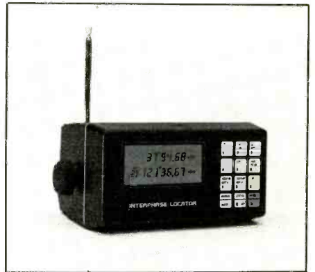
A portable Loran receiver priced at $300.
