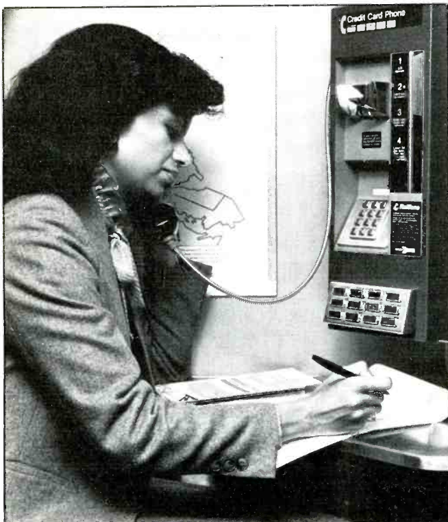
◆ GTE Railfone is the system used for placing calls from passenger trains. This provides direct-dial service through cellular base stations.
