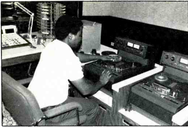
A producer in one of LRCN's Monrovia studios prepares a tape for relay to the rural stations via the ISB transmitter. The control board and a rack for cartridge tapes is on the left.
