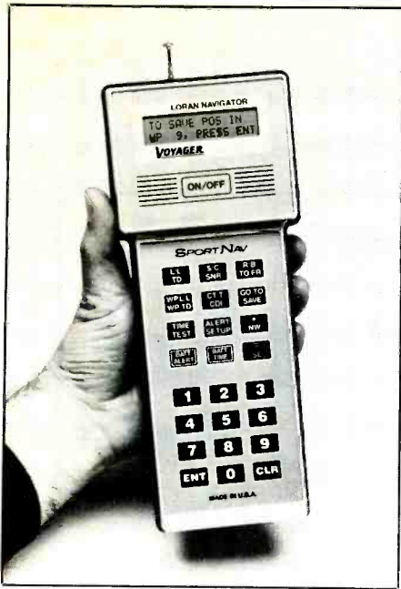
Hand-held portable, $600 Loran receiver capable of 50 foot return repeatability of your position.
