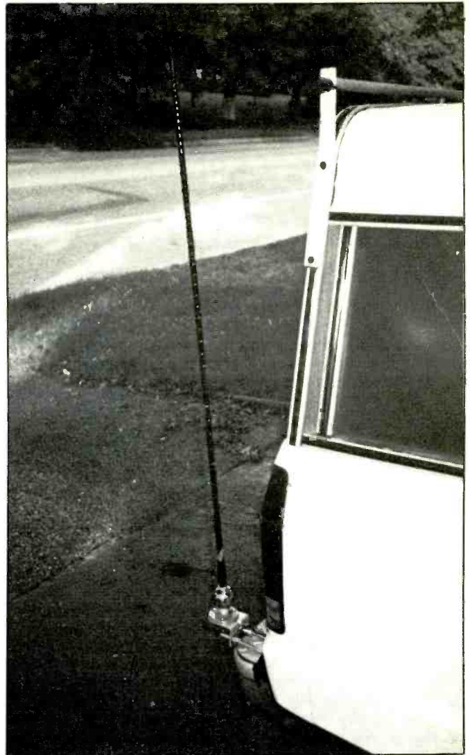
The TS-680s installed in the truck with the MFJ-204B, the switch, and the tuner. After finding and recording the tuner settings for all the frequencies you will be using, the MFJ-204B and the switch can be removed from the set up.
