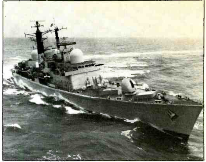
HMS GLOUCESTER (D96), one of the 'Batch three Type 42' destroyers coming off a hard turn; note the extra anchor on the fore-deck below the bridge. (Photo courtesy British Royal Navy)
