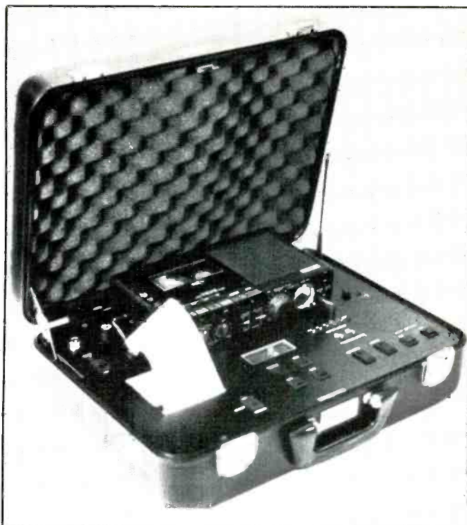
The TC-1000 eavesdrops on both sides of the suspect's telephone conversation. It also keeps a file of the numbers called along with the date and time of the call. Information can be fed to the TC-1000 by means of a small concealed radio transceiver. (Courtesy Surveillance Technology Group.)
