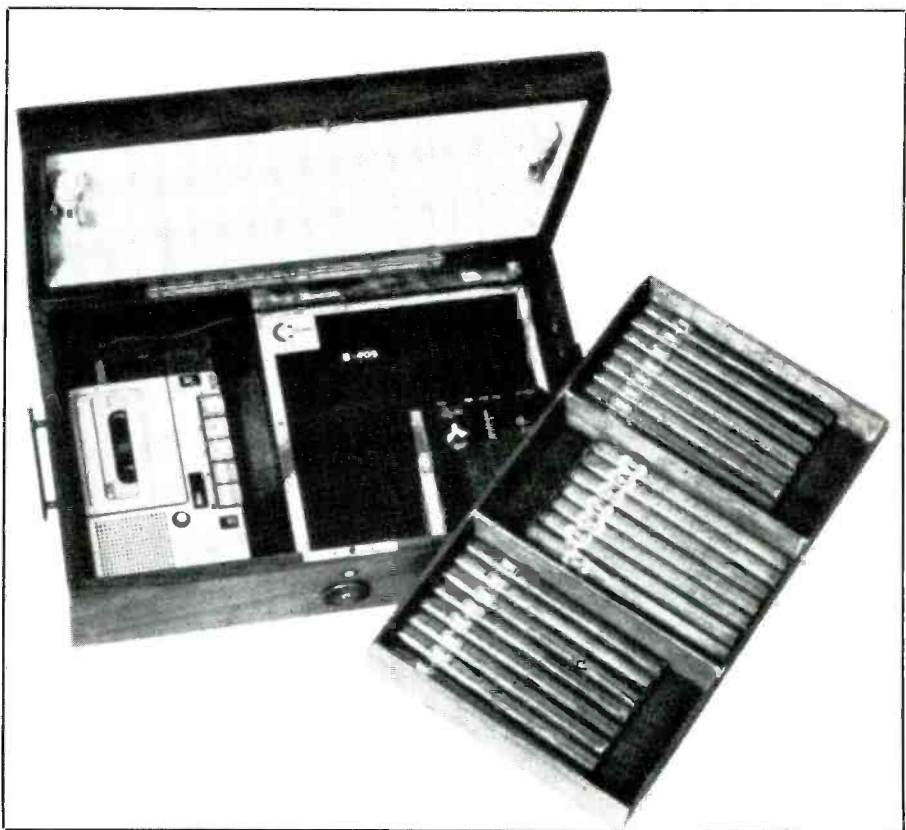
The desktop cigar humidor looks impressive, but lift off the top tray of cigars and it reveals a VOX-controlled tape recorder that picks up voices in the room as well as recording telephone calls. It also detects any concealed body transmitters being worn in the room. (Courtesy CCS Communication Control, Inc.)
