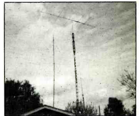
Frank Miranda's roof has a Moonraker 6, an Astron 99, an A/S M-344, and a Realistic scanner GP.
