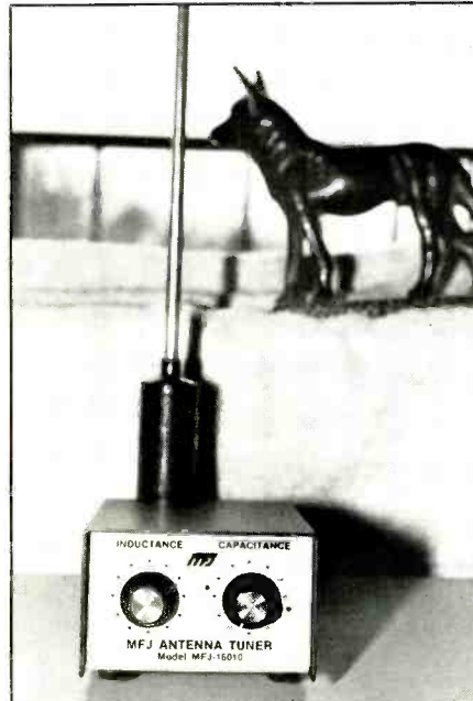
Fig 1. MFJ random-wire ham tuner peaks SWB reception when using a short indoor antenna.
