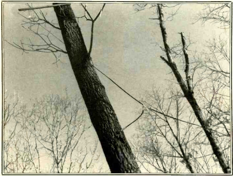
A simple wire antenna in a tree provides performance that is close to the expensive commercial designs.
