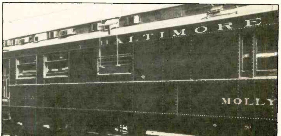
The dining car that was converted into a rolling radio station. Note the antenna on the roof and the two lead-in wires at the center window.
