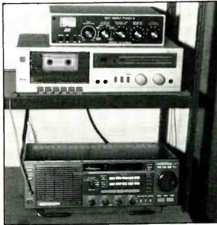
Fig. 1. Set-up for checking out ham tuner on shortwave receiver. Cassette recorder may be useful for clarity evaluation.
