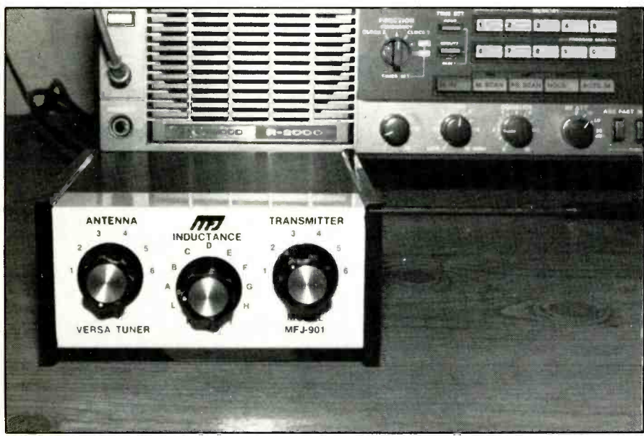
Fig. 4. Simple no-frills ham tuner can perk-up short indoor antenna wire results.
