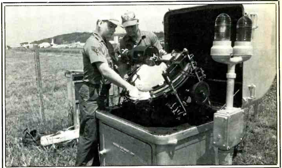
Weather equipment Technician Sgt. Edward J. Mazzei cleans the mirror of a GMQ-13 cloud height set, with the assistance of Navigational Aids Technician, Sgt. Michael R. Lilley. (U.S. Air Force photo by Capt. M.A. Gutridge.)
