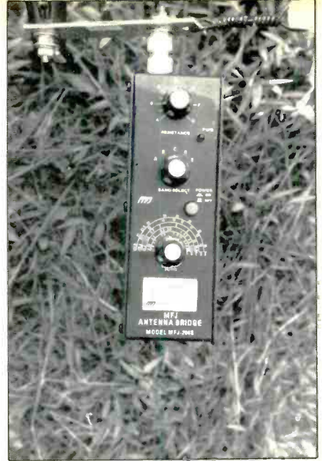
Figure 6: Antenna bridge at work.
