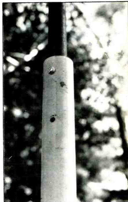
Figure 2: TV mast radiator inserted into 1/2" OD plastic pipe.
