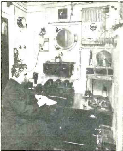
A ship's wireless "shack" in the early days of telegraphy looked like this. The "sparks" weren't part of the crew, but were employees of the Marconi Company. The spark gap transmitter is on the shelf to the right. The receiver is at the center of the operating desk.
