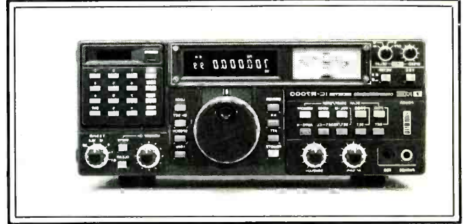
The ICOM R-7000 is an all-band scanner that tunes to 1300 MHz.
