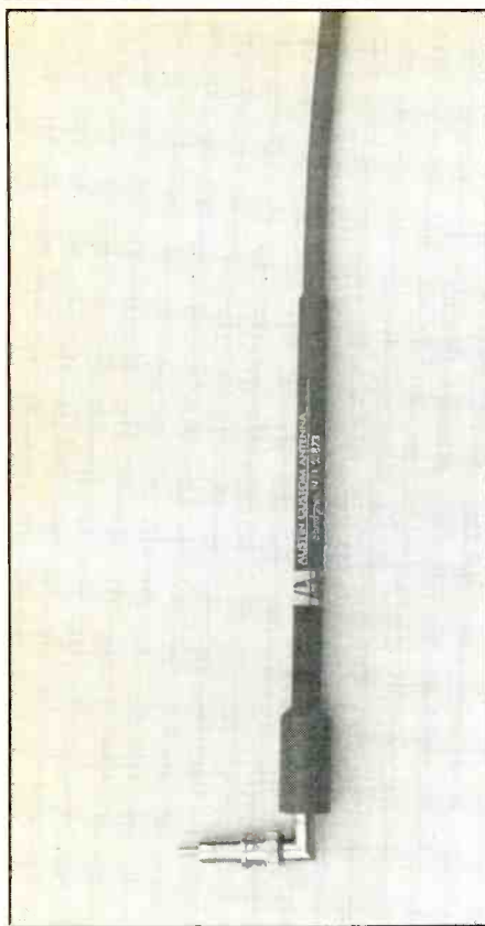
Figure 6: Elbow assembly for connecting directly to scanner.
