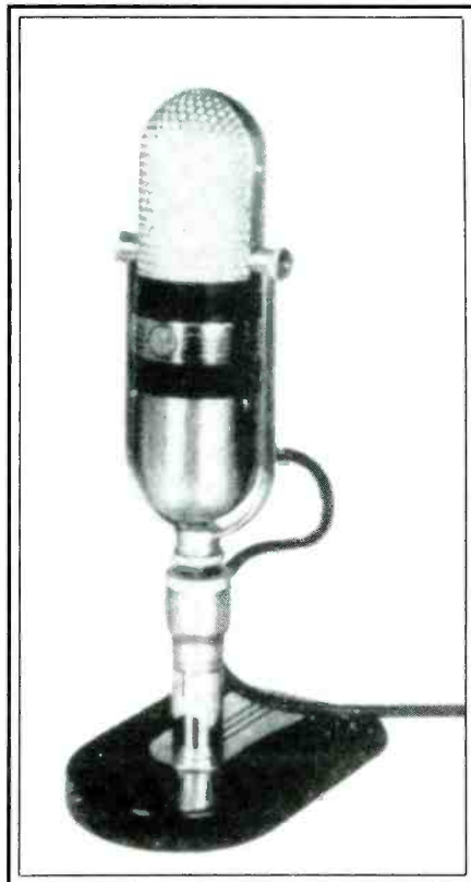
The venerable RCA Model 77D polydirectional velocity-type broadcast microphone. Would Hams and CB'ers want a reborn version in their shacks?
