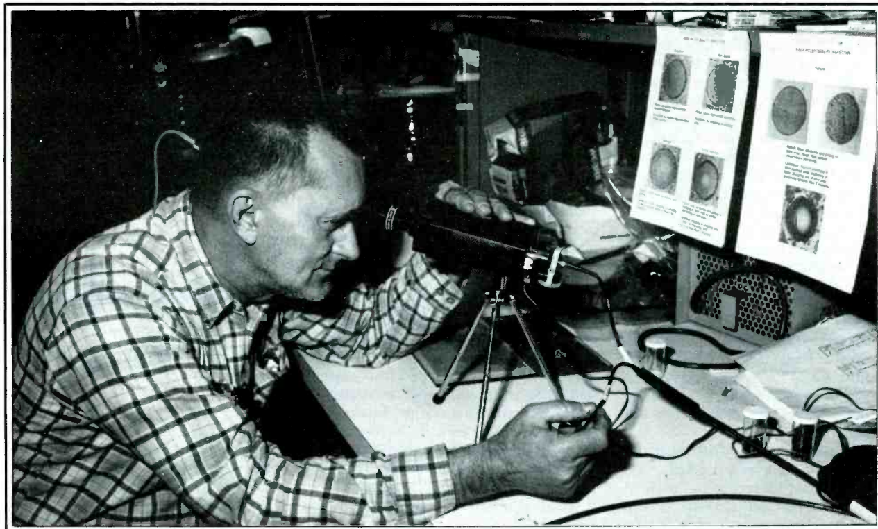
Tobyhanna Army Depot technician Joseph Bronack, peers into a microscope to inspect the polished end of a fiber-optics cable. Tobyhanna personnel recently completed the depot's first production of fiber-optics gear. It was the first practical demonstration of the depot's capabilities with fiber-optics technology, which offers several advantages over standard electrical cables. (U.S. Army photo.)
