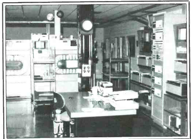
It's hard to visualize just how large a metro TV station is. These two photos show about half of the video tape area at WBAL-TV. If you look beyond the desk in the center of the left photo you see the window and doors leading to the control room seen in the film Diner. The big brutes with the ovals in the center (right photo) are TV cartridge machines. To the right are many cassette machines used, among other duties, to play the cut-ins on newscasts. The station has about 20 tape machines in this area.
