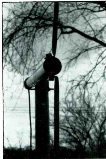
Figure 3: Bolt/nut terminals for attaching antenna elements and line.
