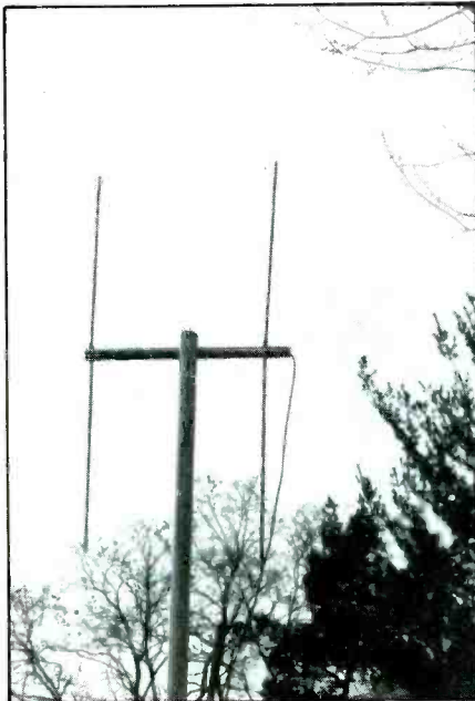
Figure 5: Aeroband two-element beam.
