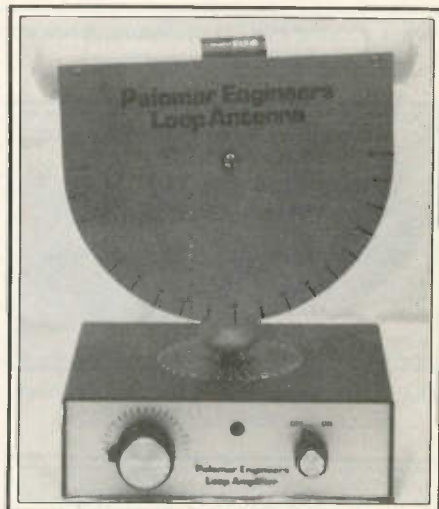
This indoor loop antenna and amplifier can save you the trouble of stringing a long wire antenna.
