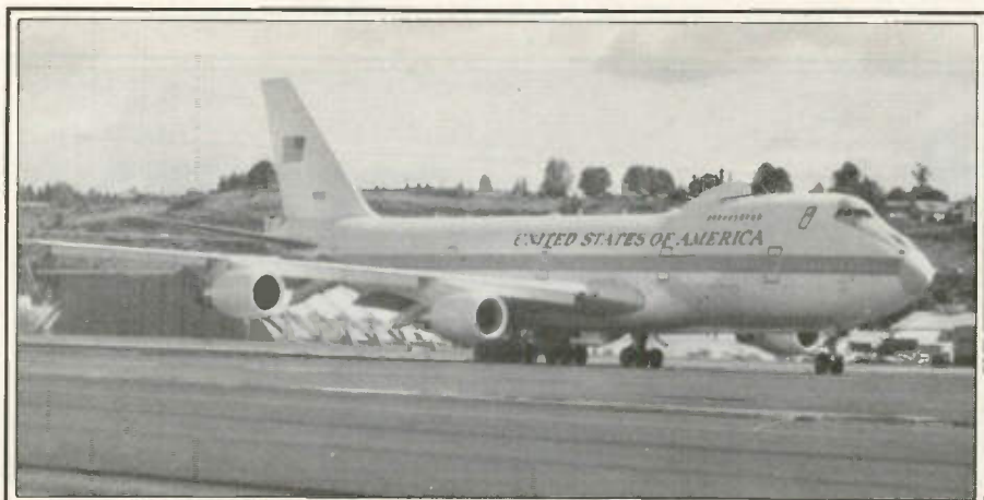
The USAF AABNCP can fly for up to 72 hours during a national emergency. It has VLF communications facilities.
