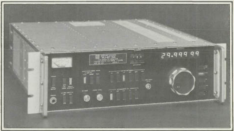
A very sophisticated, modern receiver covering these frequencies is the Watkins-Johnson Company's WJ-8718A. It covers 5 kHz to 30 MHz in all modes.
