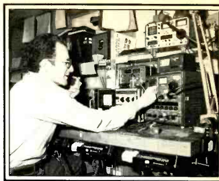
Alvin Solomon of the NYPD checks the frequency and deviation of a transmitter.
