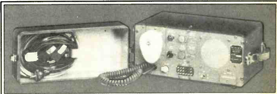
The TR-20's transmitter used "instant heating" filament type tubes in both the PA and oscillator/tripler stages. The transmitter's modulator and power supply was transistorized, as was the complete receiver circuitry.
