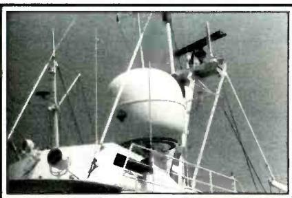
A marine SATCOM antenna system.
