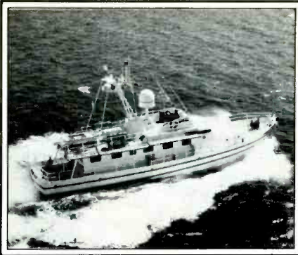
Now type approved by INMARSAT, the Magnavox MX 211A Ship Earth Station with its distinctive new small antenna as installed on the MV Duchess Diane.
