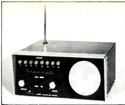
Electra's early scanner. It had only 8 channels, no lockouts, no delay, no search or scan-speed features. The public loved it anyway and it opened the door for modern PSB monitoring.
