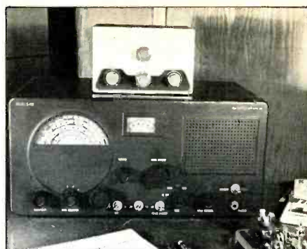
In the early days of PSB monitoring, it was necessary to use a communications receiver which tuned up to the VHF low band, like this Hallicrafters S-40B.
