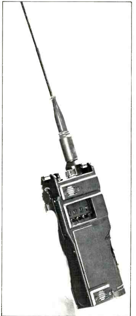
The PRC-613 and PRC-614 are palm-held VHF-FM radios covering 33 to 53 MHz and 53 to 76 MHz respectively in 25 kHz steps. Both employ digital frequency synthesizer controlled by miniature pushbuttons. They feature advanced circuitry and thick-film modules using monolithic IC's. One WRF output. Developed by Tadiran.
