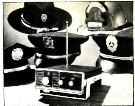
Later refinements in circuitry permitted Regency to produce this 6-channel solid-state receiver.
