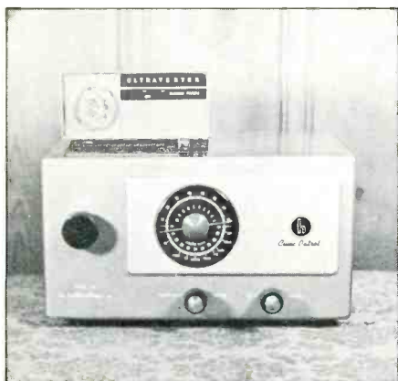
Hallicrafters' venerable Civic Patrol receiver (shown in use with a UHF converter.)
