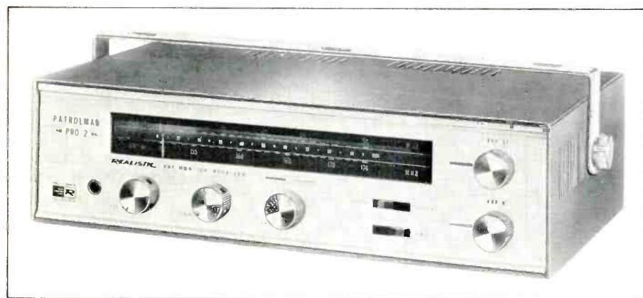
Radio Shack's PRO-2 was an early tunable PSB receiver which covered the hi and lo VHF bands. It was a solid-state receiver.
