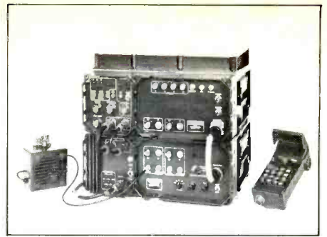
Advanced direction finding system for tactical applications, operating on the principles of interferometry and notable for high accuracy, quick response, and processing capability. The TDF-3090 may be used independently or as an integral part of a large COMINT system. It is suitable for installation in mobile shelters, APC's, small naval craft, and other vehicles. Modems are available for high-speed data transmission via radio or wire. This equipment is produced by Tadiran, Israel Electronics Industries Ltd.
