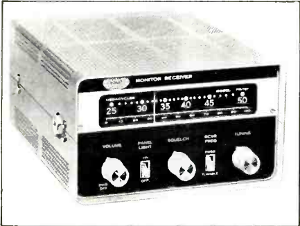
Sonar was an early hopeful in the PSB monitoring sweepstakes. This is one of their first tunable receivers, the FR-101, which had a crystal for single frequency reception.
