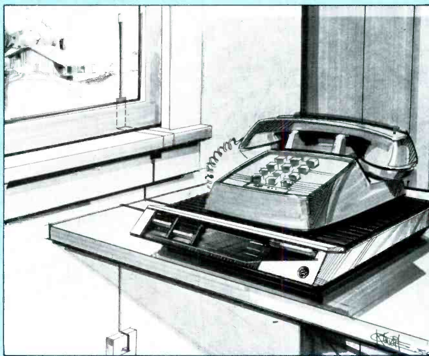
The PRCS base station will be interconnected to the telephone lines and will give the motorist a chance to place calls directly through his own facilities.
