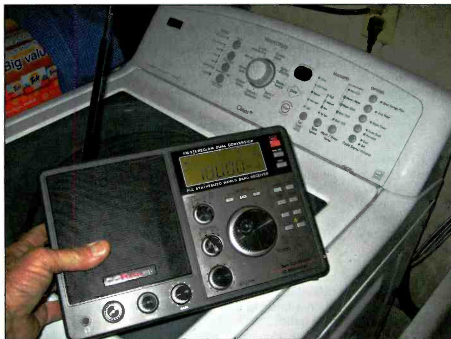
Photo D. This clothes washer put out so much RF it could work DX on 40 meters. The solution was to put it under house arrest — shut it off — when operating on the 7-MHz band.
