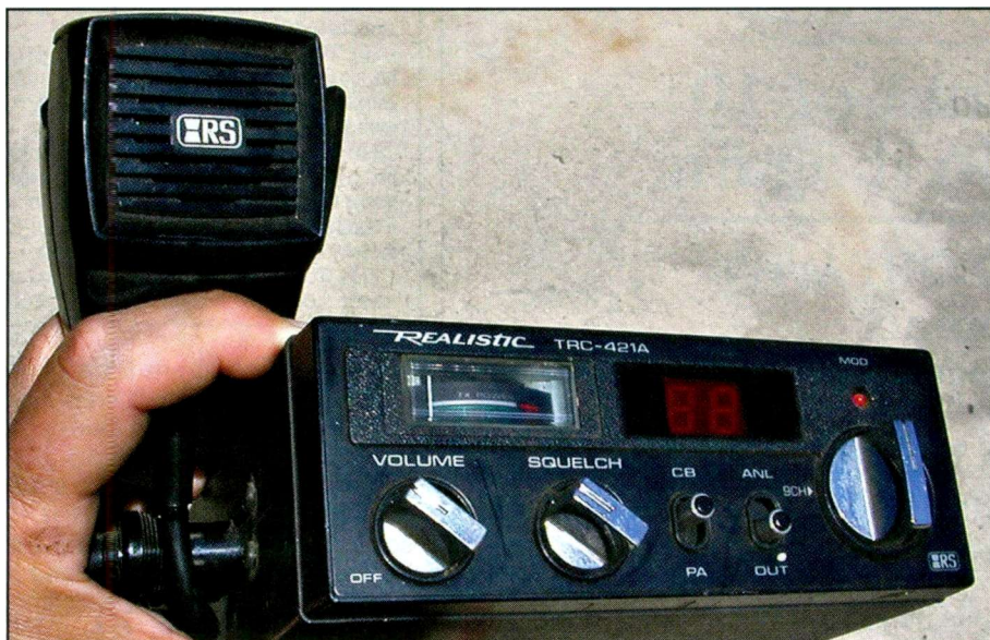
Photo A. Used CB radios, such as this 40-channel Realistic TRC-421A AM transceiver, are selling today for well under $25 on auction sites such as eBay. (Courtesy of KPC6PC)
