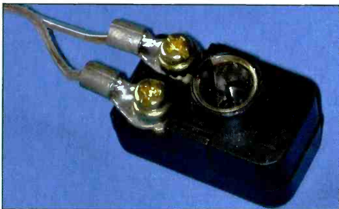
Photo E. Solder lugs on the receiver-end of the feed line were connected to a standard antenna adapter (RadioShack® 15-1253 or similar) to make connecting to the KPC6PC Wave Radio a snap.
