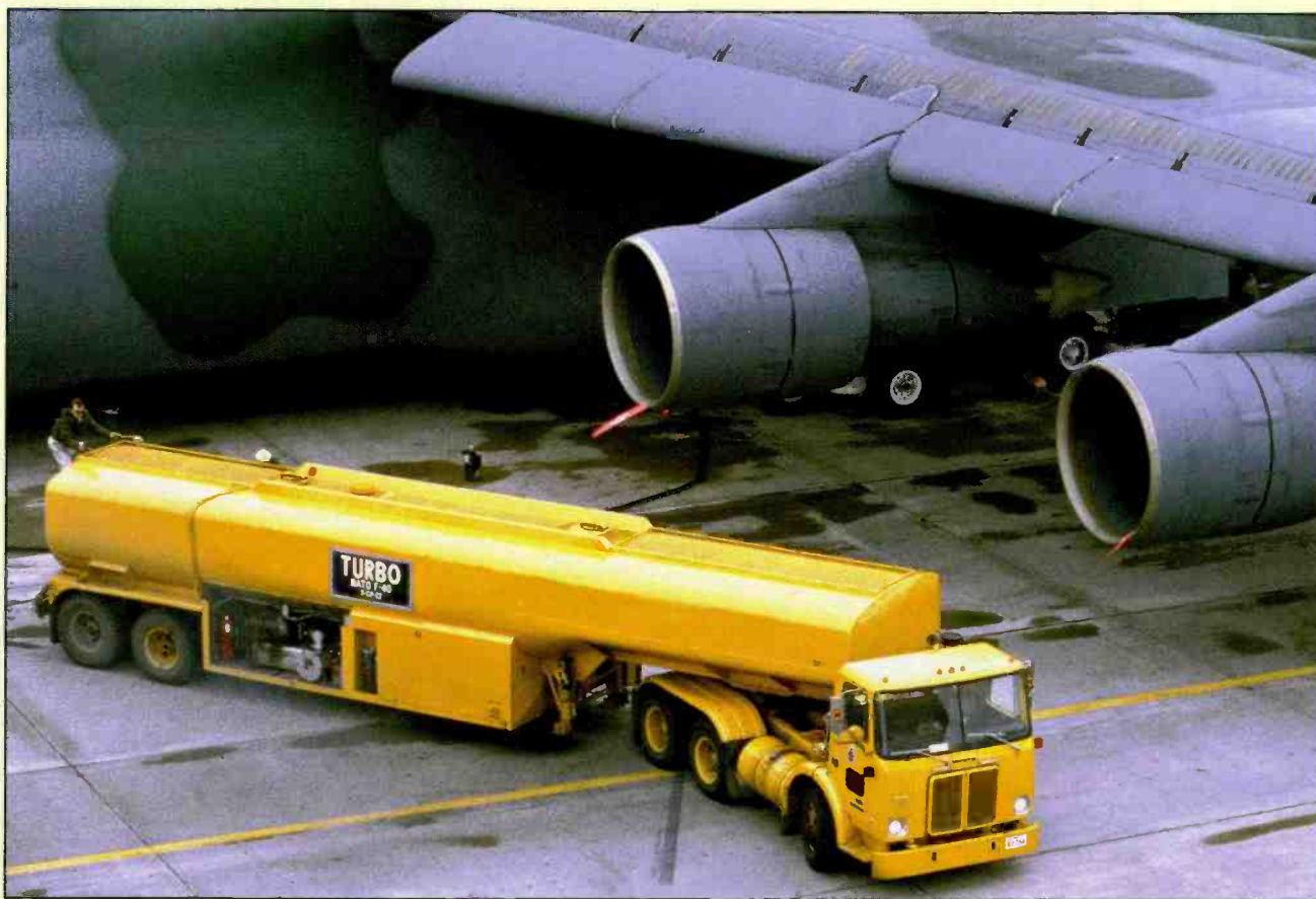
Photo H. A large aviation fuel truck is dwarfed by the giant C-5A Galaxy — one of the largest aircraft in the world. The horizontal stabilizer is larger than some commercial jets' wingspan, and the aircraft is so big, it produces two blips on controllers' RADAR. (Courtesy of Wikimedia Commons)
