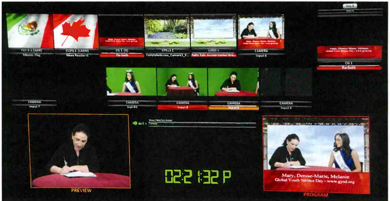
Photo E. The main monitor in the control room displays the three camera inputs with green backgrounds, along with overlays, graphics, and the final program channel with chroma key effects.
