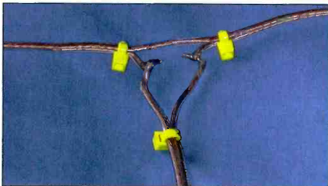
Photo D. This mini-pictorial shows how the feed line is soldered to each side of the horizontal folded dipole, and where zip ties were added to keep the wires from further separating.
