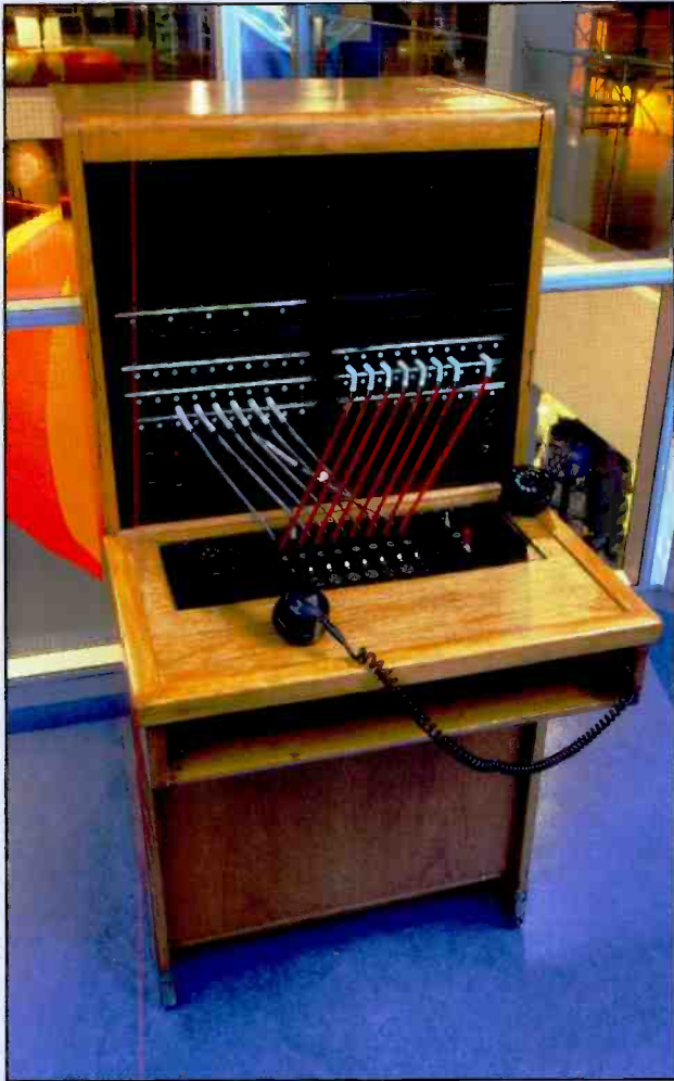
Photo F. This classic PBX switchboard shows the color-coded cables, used by its operator to keep track of which calls were going where. (Courtesy of Wikimedia Commons)
