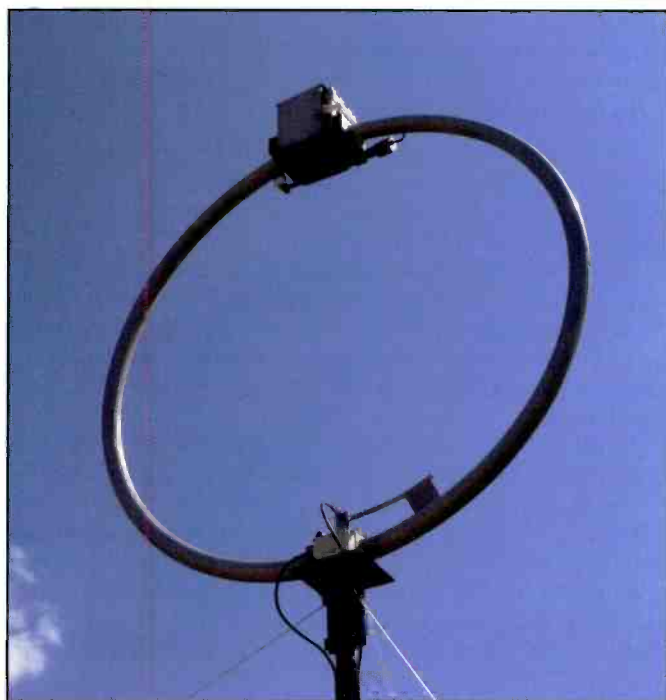
Photo C. Loop antennas can be an ally in fighting noise. This vertical loop covers 1.75 through 30 MHz with its automatic tuning unit. WPC7USA recommends a 160-foot-long, horizontal loop as a quiet and effective antenna — if you have the room. See text for details. (Courtesy of ©Trix via Wikimedia Commons)
