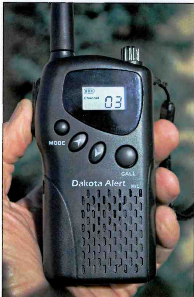
Photo B. This MURS handheld transceiver runs 2 watts with a bank of AA batteries. (Courtesy of WPC6NOA)
