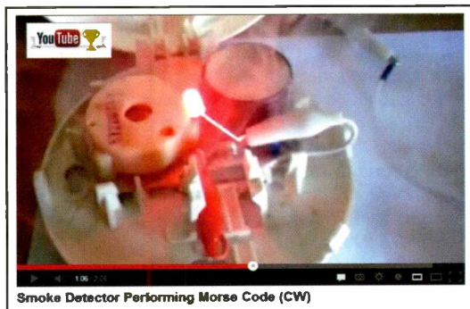
Photo B. With an assist from an Arduino electronics prototyping platform, Luther Banks, KD8NCL, gets a smoke detector to send his amateur radio callsign in Morse code. (Internet screen grab < http://bit.ly/11d4RyT >.)
