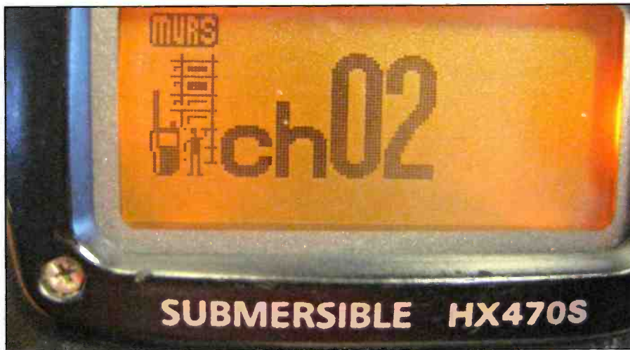
Photo E. Monitors can listen to MURS channels using various receivers. This marine radio handheld is tuned to MURS Channel 2. (Courtesy of WPC6NOA)
