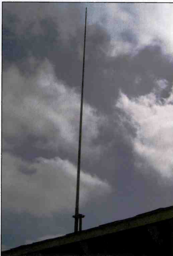
Photo C. This VHF collinear array will give the MURS operator 9 dB of gain at a base station — a considerable advantage over 2 watts going into a small whip antenna. (Courtesy of WPC6NOA)
