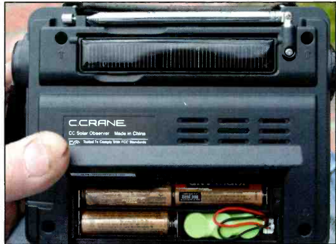
Photo E. On the rear side of the C. Crane Solar Observer, users find the radio's solar panel and battery compartment. They are among a slew of power options.
