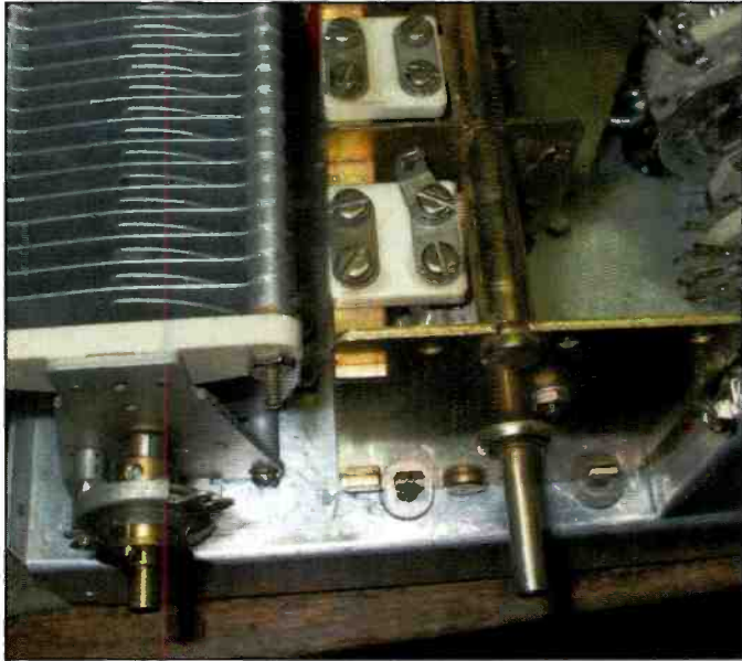
Photo G. A Jackson Brothers vernier reduction drive was added to the plate tuning capacitor for easier plate tuning on the higher HF bands.
