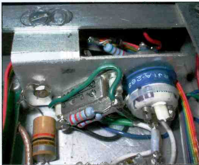
Photo D. These are the RF antenna changeover relays. The high-power RF switching uses a very fast vacuum relay for true QSK CW.
