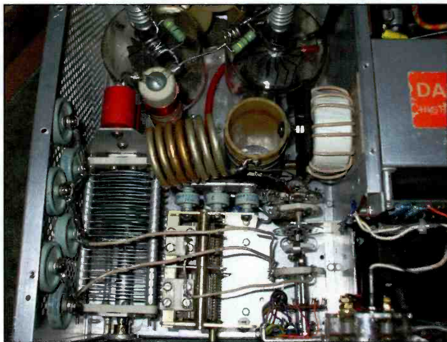
Photo F. Take a look at the new RF deck. Adding 160 meters and the WARC bands required an extensive redesign of the entire PA network!
