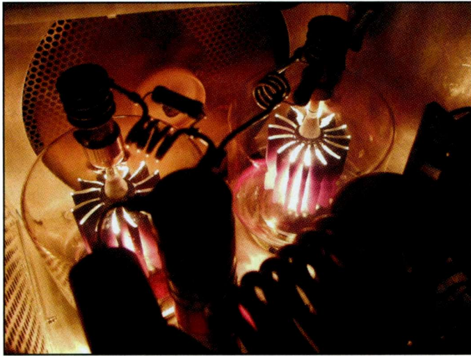
Photo I. Keep those old tubes glowing! The 3-500Z final tubes are getting a work out on 160 meters. That red plate glow is a good thing. It helps keep the tubes gettered and degassed.
