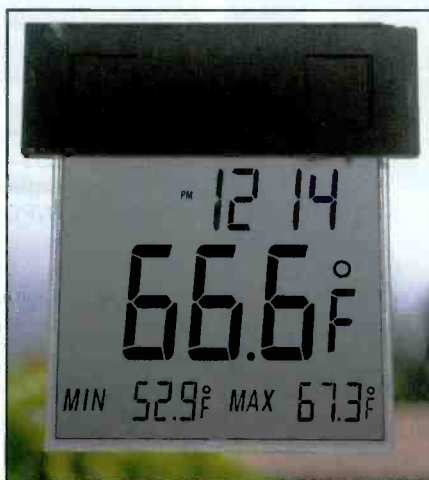
Photo H. La Crosse Technology's solar-powered window time-and-thermometer's translucent display is illuminated by two LEDs, which get charged via a tiny solar panel during the day.
