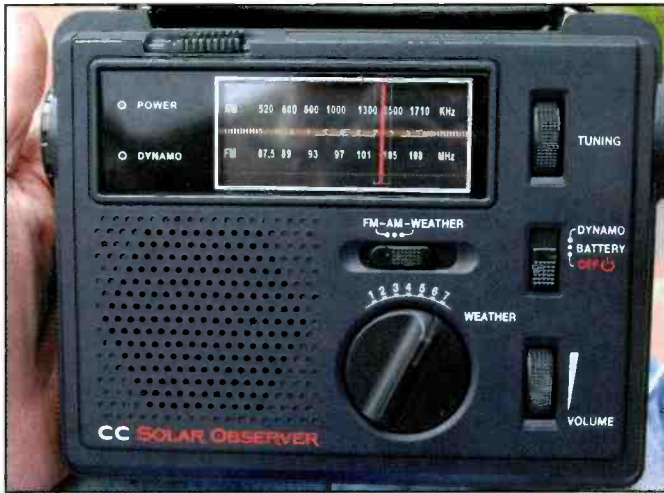
Photo D. The C. Crane Solar Observer features AM/FM radio reception, plus seven weather channels. For power, it has a hand-crank dynamo power generator, solar power generation, regular AA battery power, and a rechargeable power pack. It can charge cell phones, as well.
