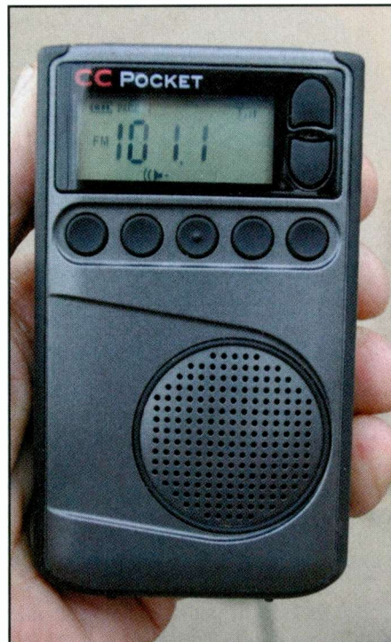
Photo C. The C.Crane CC Pocket receiver is an AM/FM stereo receiver featuring narrowband AM and a weather alert function. Also: a clock, auto off, and an alarm. “Great audio!” says WPC6NOA. “Very compact and great reception with stereo top-quality earphones included.”
