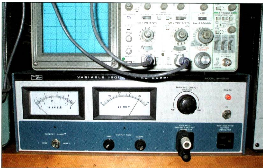
Photo A. The author’s Heath SP-5220 combines a variac , isolation transformer, fused output, and full current and voltage metering in one compact package. (Photography by K1ZJH)
