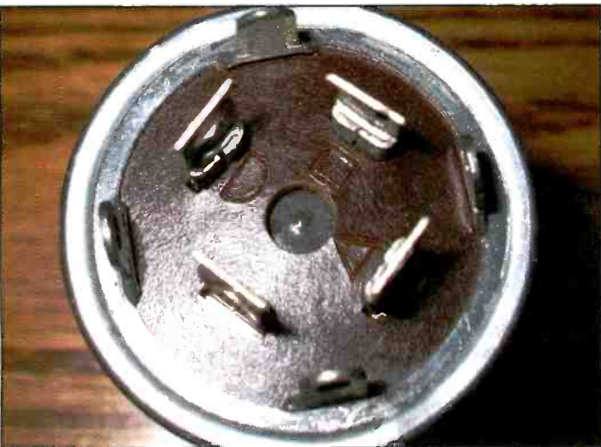
Photo F. The symbols for the various sections are embossed on the insulation material for this four-section capacitor.
