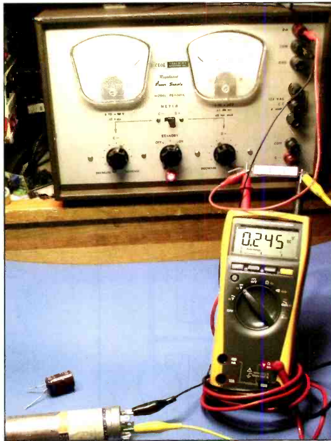
Photo C. The author's Stark variable DC supply, along with a Fluke 177 digital meter, is used in this test setup which measures NOS electrolytic leakage currents. The Sprague NOS electrolytic capacitor is showing less than 50 \mu\text{A} at near-rated operating voltage.
