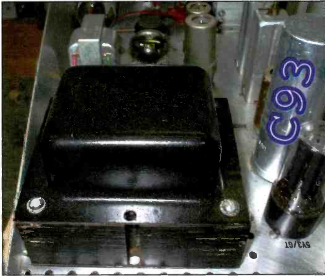
Photo D. Location of the three-section main filter capacitor on the SX-101A chassis. This is capacitor C93.
