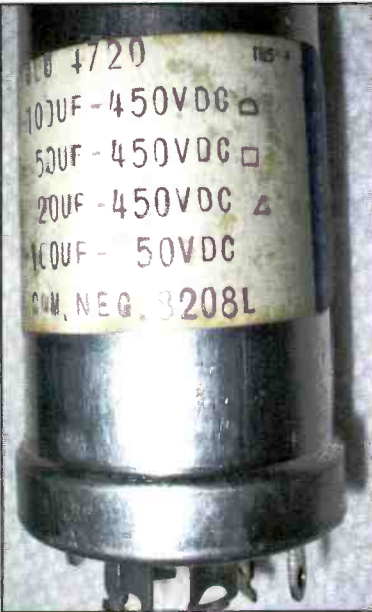
Photo D. Location of the three-section main filter capacitor on the SX-101A chassis. This is capacitor C93.
