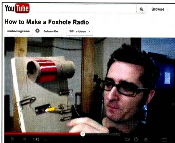
Photo A. World renowned maker Bre Pettis shows how to make an authentic foxhole radio — razor blade and all, < http://bit.ly/Q2J7zV >. (Internet screen grab)
