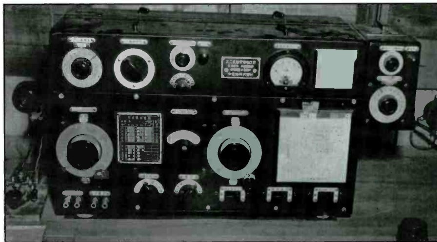
Photo E. Here is a panel view of a Japanese radio transmitter/receiver after it was put back on the air by U.S. Marines. Note the key to the left of the set. The Japanese equipment was largely copied from American designs. It was efficient, substantially built and had surprising power and range.
