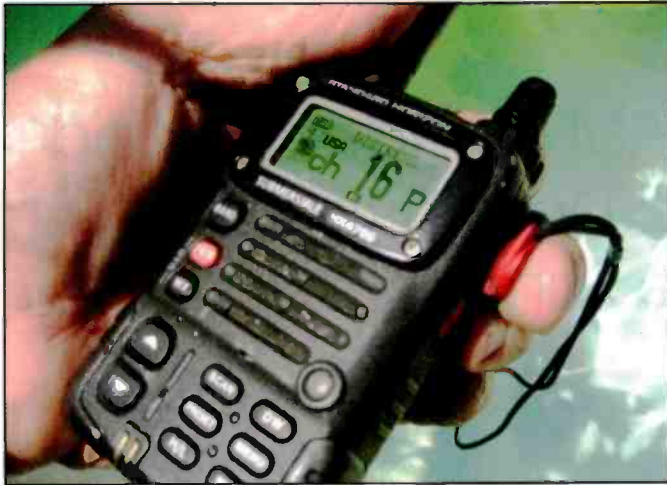
Photo H. A handheld marine VHF radio is a great way to check modulation over the air. Wiggle the microphone cord, too, to check for a solid connection.
