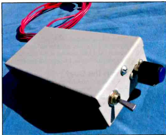
Photo C. An ON/OFF toggle switch and knob for the VPA's 50-pF tuning capacitor are positioned on the front panel.
