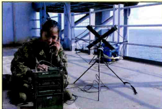
Photo I. Marine Lance Corporal Christine Salazar of the 24 th Marine Expeditionary Unit, uses a PRC-117 and SATCOM antenna to receive satellite communications. (Courtesy of U.S. Marine Corps)
