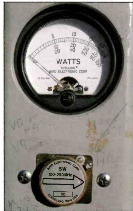
Photo C. You will need a professional watt meter to conduct power output checks during radio inspections with the GROL license.
