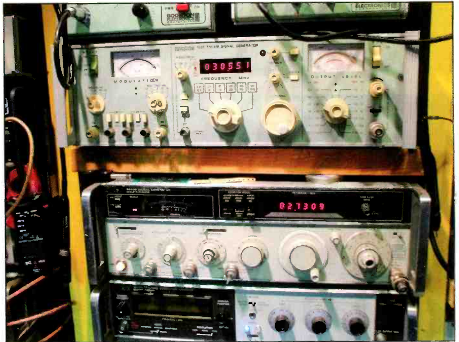
Photo J. The Boonton 102F, and the HP 8640B below it, are the best generators I own. Although the 8640B generators are nearing, or past, their sunset years, they can be kept running thanks to the availability of parts from donor units.
