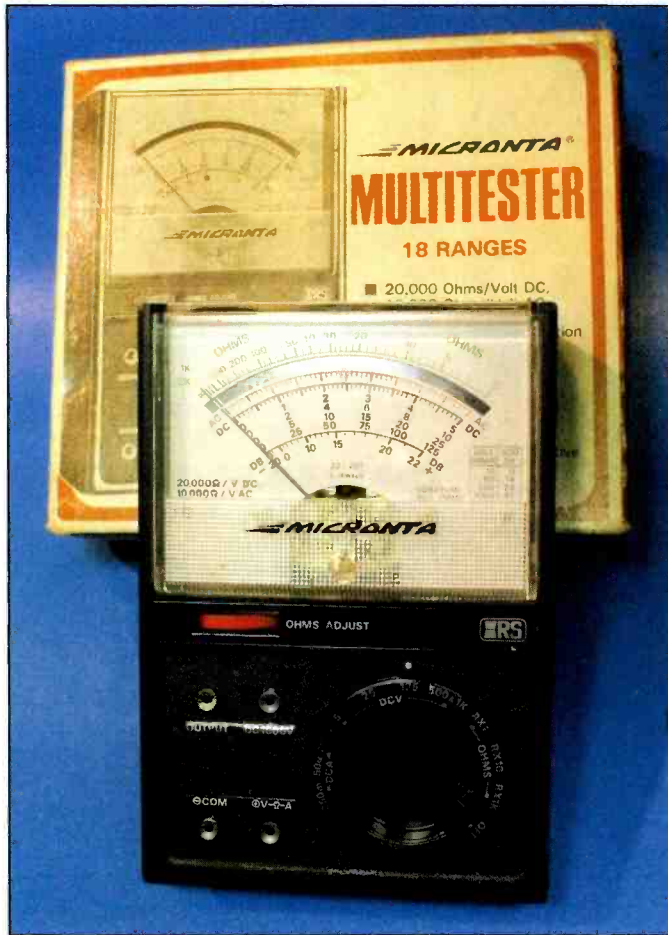
Photo F. Here's a 1975 vintage RadioShack® Micronta Model 22-201 volt ohmmeter. It was an inexpensive yard sale find, but it will do the job for a beginning electronics hobbyist!
