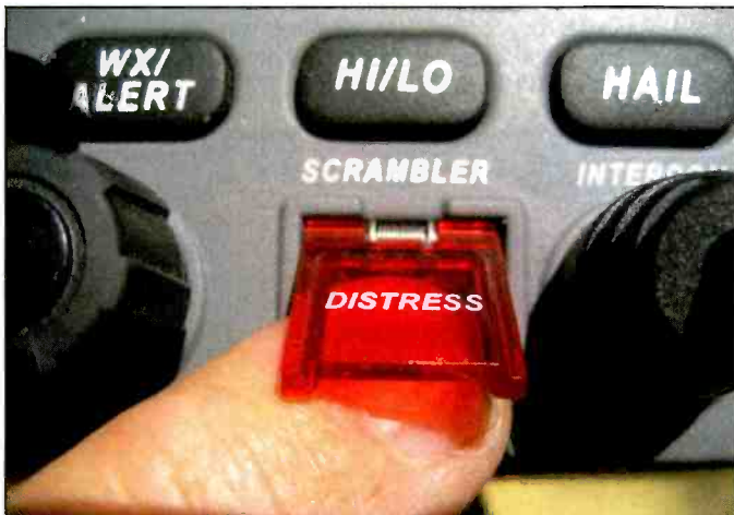
Photo 1. Digital Selective Calling is now an integral part of marine VHF transceivers. You can spot a marine VHF radio with DSC capability by the red plastic cover over the hot button. The red plastic cover is spring-loaded to prevent an accidental activation.
