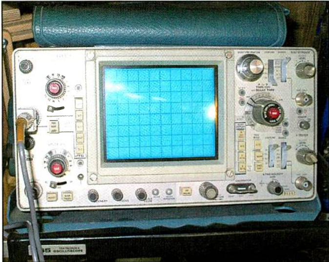
Photo N. The Tektronix 465 arrived in my shop about 30 years ago. The 465 was extremely popular and well respected scope. I probably have too many scopes!
