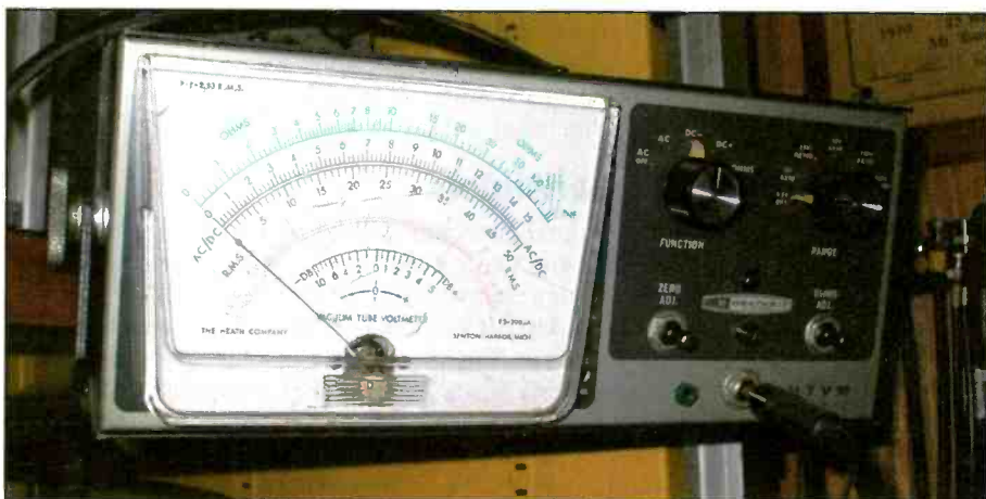
Photo E. My Heathkit IM-28 VTVM comes in handy when an analog meter is needed for alignments.
