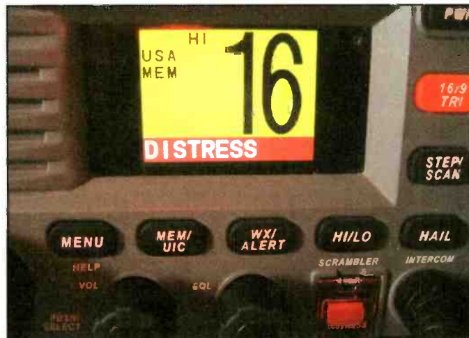
Photo C. Harbor Patrol, Lifeguard, Sheriff's Department, Lake and Rescue 21 base stations and patrol vessels monitor VHF channel 16.
