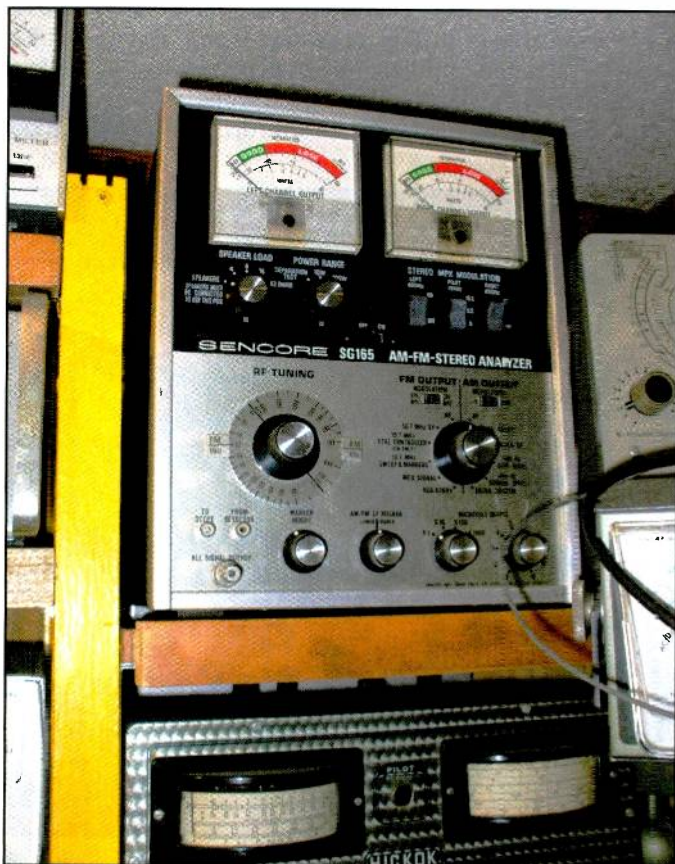
Photo I. The Sencore Model 165 signal generator covers the AM and FM bands, and features a FM stereo modulator.
