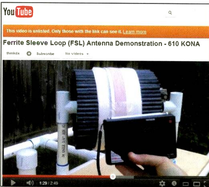
Photo E. Watch video of Gary DeBock demonstrating a ferrite sleeve loop antenna used with a Tecsun PL-380 receiver at < http://bit.ly/1lfhpiy >. (Courtesy of Gary DeBock)
