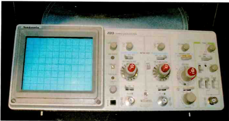
Photo L. I picked up this Tektronix 2213 scope 10 years ago for around $50 at a tag sale. It is a dual channel, 60-MHz scope with triggered sweep. The 2213 is a good basic scope for beginners. It lacks delayed sweep, which keeps the price way down!
