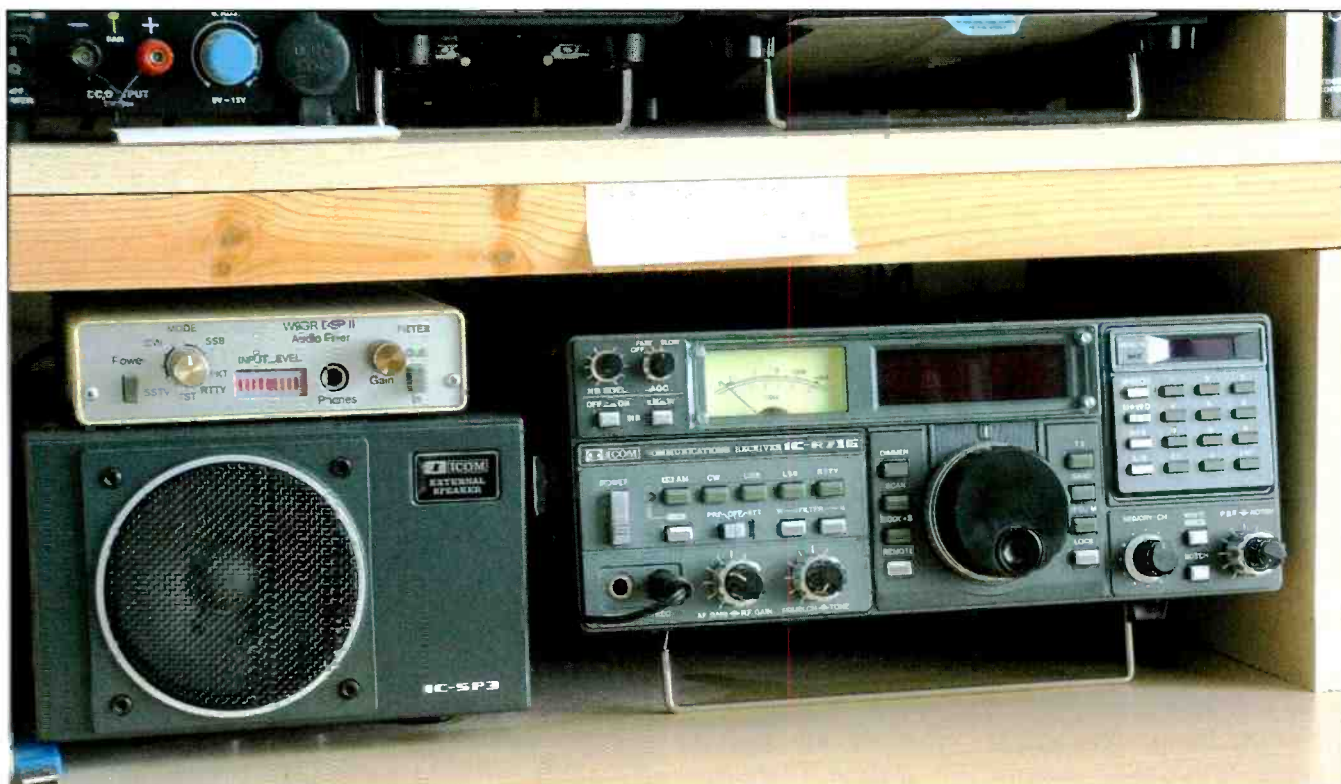
Photo E. A close-up view of GPCØAB's ICOM IC-R71E receiver and matching IC-SP3 speaker show only part of the beauty of the gear at his island listening post.
