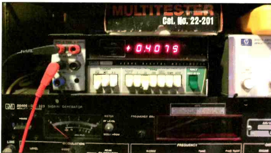
Photo D. The Fluke 8800A digital voltmeter is a bench model and runs on AC power.
