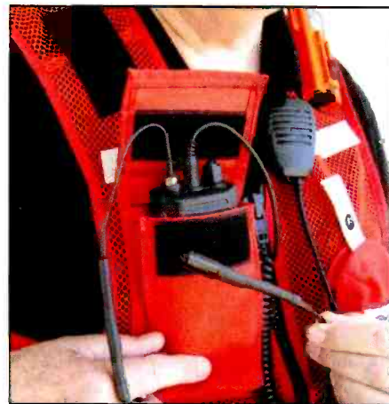
Photo G. New marine handheld radios are submersible and easily fit in a Personal Flotation Device pocket — just in case you go overboard.
