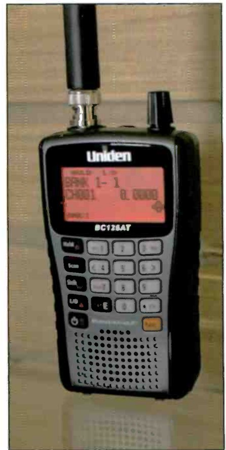
Photo L. The Bearcat BC125AT scanner by Uniden® features 500 channels with a wide range of frequency coverage: 25-54, 108-174, 225-380, and 400-512 MHz.
