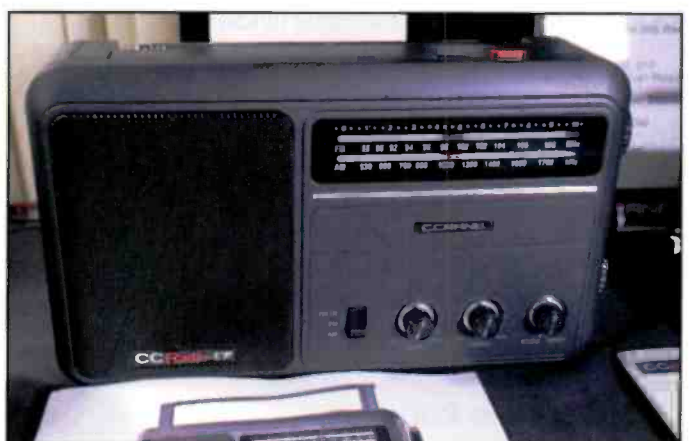
Photo S. The CCRadio-EP, with twin coil ferrite antennas built in, takes "the directionality out of a portable receiver" while allowing the twin antenna system to be fine-tuned to cancel out interference. It's by C.Crane Co.®
