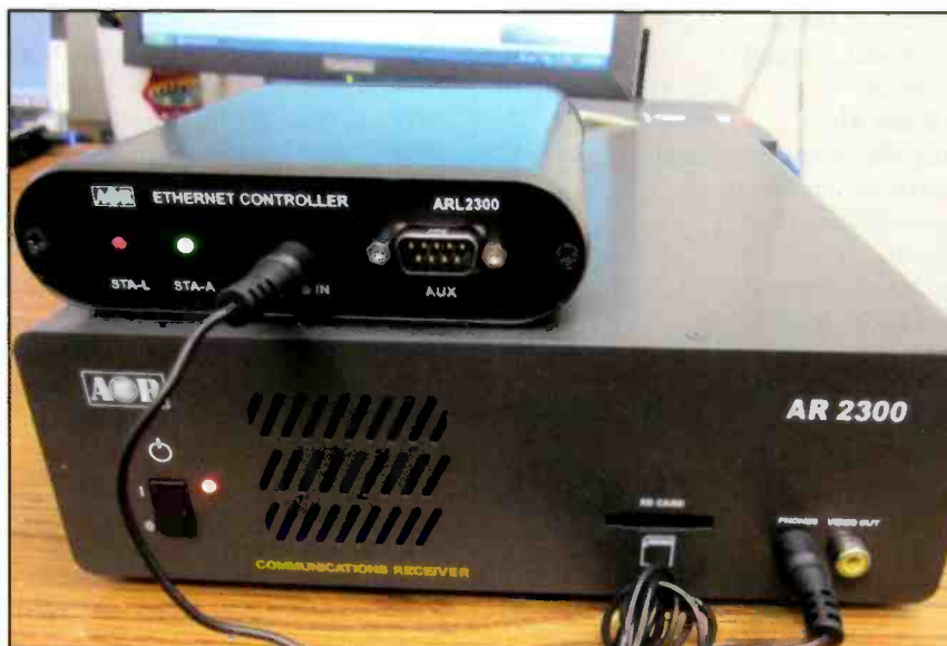
Photo A. The AOR ARL2300 Ethernet Controller provides connections for either the AR 2300 (shown) or the AR 5001D receiver and interfaces it to the Internet via the Ethernet. (Courtesy of AOR)
