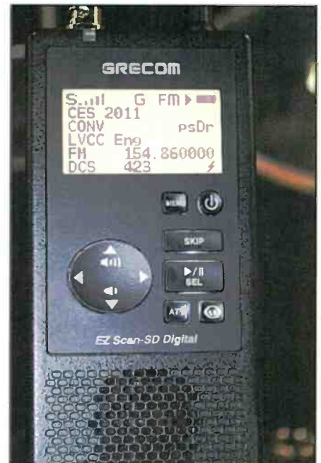
Photo D. The GRE® PSR-800 EZ Scan Digital P25 Scanner is an HT-sized trunking receiver that is "nearly self-programmable."
