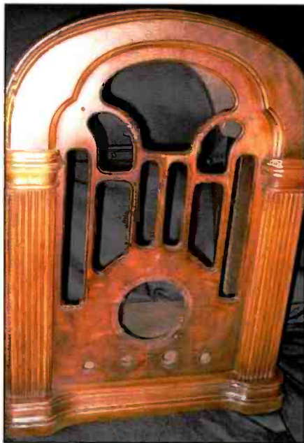
Photo J. After smoothing the wood, "I have seen many people who reach this stage, say, 'Wow, that's beautiful,'" Mornhinweg, writes, and then "spray on a coat of clear lacquer, and assemble the radio. The Web is full of such impeccably restored radios!"
