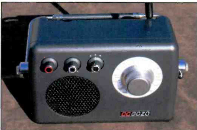
Photo R. The CC Gozo, by C.Crane Co.®, "uses conventional big capacitor analog tuning allowing the receiver to wiggle between two strong stations and pull out a weak one," writes Gordon West, WB6NOA.
