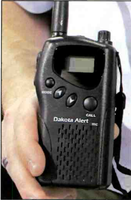
Photo H. The Dakota Alert M538-HT is a handheld MURS (multit-use radio service) transceiver “that can serve as the alert monitor for an activated sensor, or work on the five MURS channels with a similar HT.”
