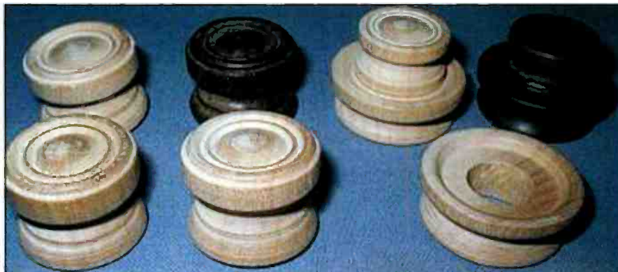
Photo B. Knobs were borrowed from an original Atwater-Kent 206-D receiver, which were used as a guide. "A humble broomstick" was sacrificed to reproduce new knobs on a lathe.
