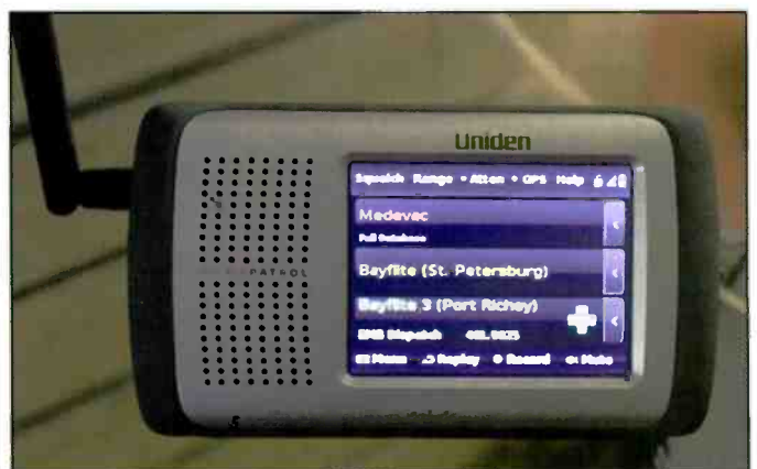
Photo G. The HOMEPATROL-1 scanner by Uniden® “includes a 2G micro SD card, and is pre-programmed with all-known U.S. and Canadian systems.”
