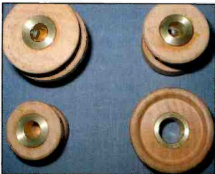
Photo C. Four different knobs are used on the AK 206-X. The band switch and tone switch knobs are replicated on the upper right. The tuning shaft is double concentric, so for the vernier drive, the lower right knob is used for fast tuning and the lower left knob is used on top of it for fine tuning. The volume control, for symmetry, uses a single knob in the same shape as the two tuning knobs combined.
