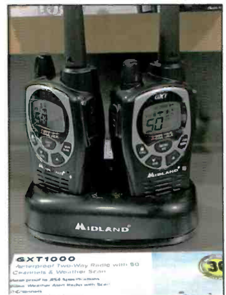
Photo M. The Midland® GXT1000 is a GMRS-FRS transceiver that is water-proof, has 50 channels and can run on either four AA alkaline batteries or an optional NiMH battery pack.
