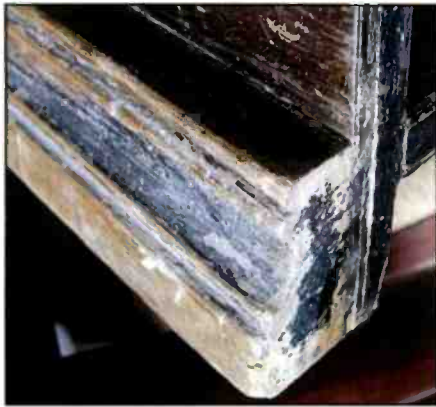
Photo E. The backside is painted black. "The stripe along the molding looks black too, while the rest is walnut brown, except where no finish is left," Mornhinweg writes. "So, was the black stripe made with the same paint used on the back? Apparently not: The paint on the back dissolves very quickly . . . while the black stripe was very slow."
