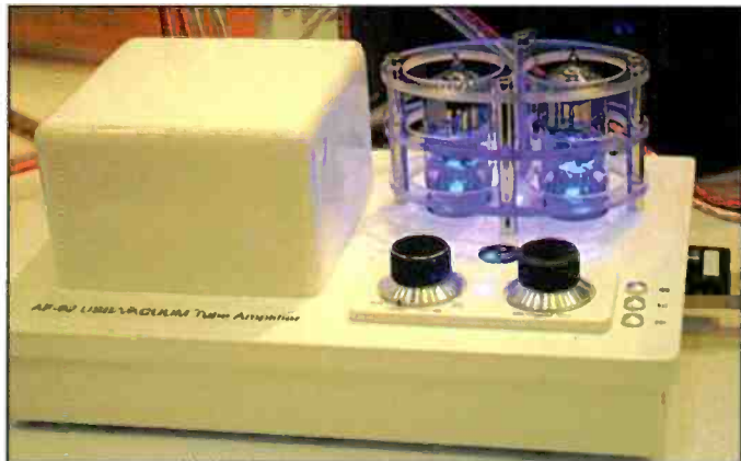
Photo W. Gordon West reminds us that tubes are not a thing of the past in big stereo systems. Check out Audio Power Labs'® 50-watt AF-02 USB/Vacuum Tube Amplifier, featuring a pair of 572B tubes.
