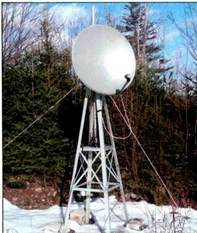
Photo E. A Ku-band dish on a six-foot-tall tower helps Murray Lycan pursue one of his other monitoring passions — satellite TV DXing.
