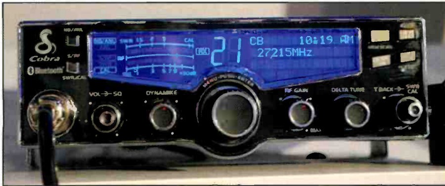
Photo N. About 15 CB transceivers were displayed by Cobra®, with its C29 allowing for integration of a Bluetooth™ cellular phone. “You hear the return audio coming from its very loud built-in or optional speaker,” WPC6NOA writes. The user has a choice of background colors on the rig’s display.
