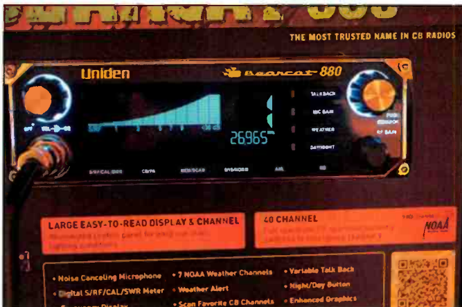
Photo J. The Bearcat 880 is among three 27-MHz Citizens Band transceivers Uniden® has added to its product line.
