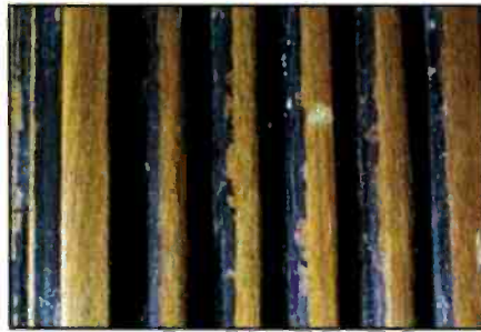
Photo G. Mornhinweg took samples from various parts of the finish, analyzed them, looked at them under different lights . . . "and it was puzzling at best." He believes Bitumen of Judea was used as a dye, and applied it both as a paste filler . . . "and mixed with the lacquer that was sprayed on."
