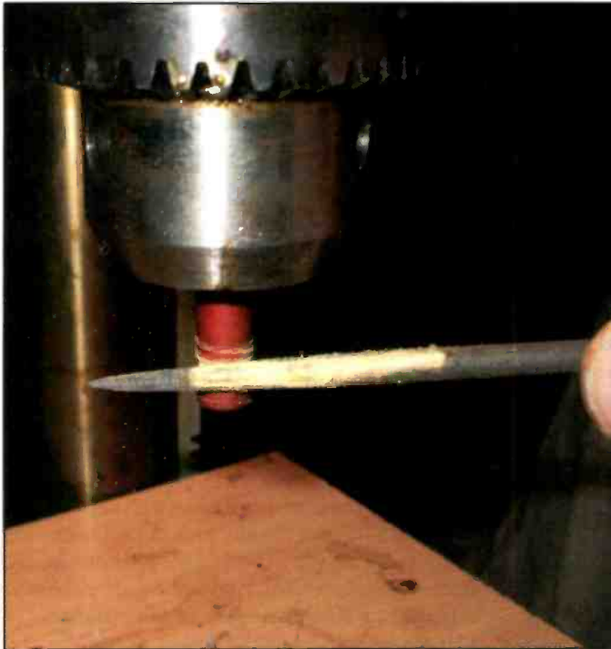
Photo G: Purists may wish to remove enough Phenolic material so the dial cord no longer rides against the standoff. This was done using a rattail file held against the standoff, as it rotated while chucked in my drill press.
