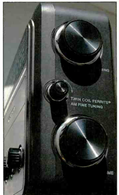
Broadcast band DX can be optimized — and QRM minimized — by adjusting the CCrane EP radio’s twin coil antenna phasing.
