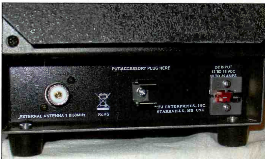
Photo H. PowerPole DC interface.
