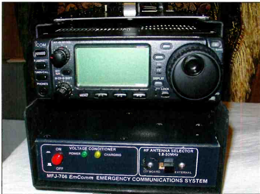
Photo C. Front view with IC-706MKII mounted. Note storage space under radio.
