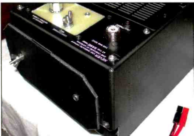
Photo K. New ground lug and stainless steel mounting screws on rear cover.
