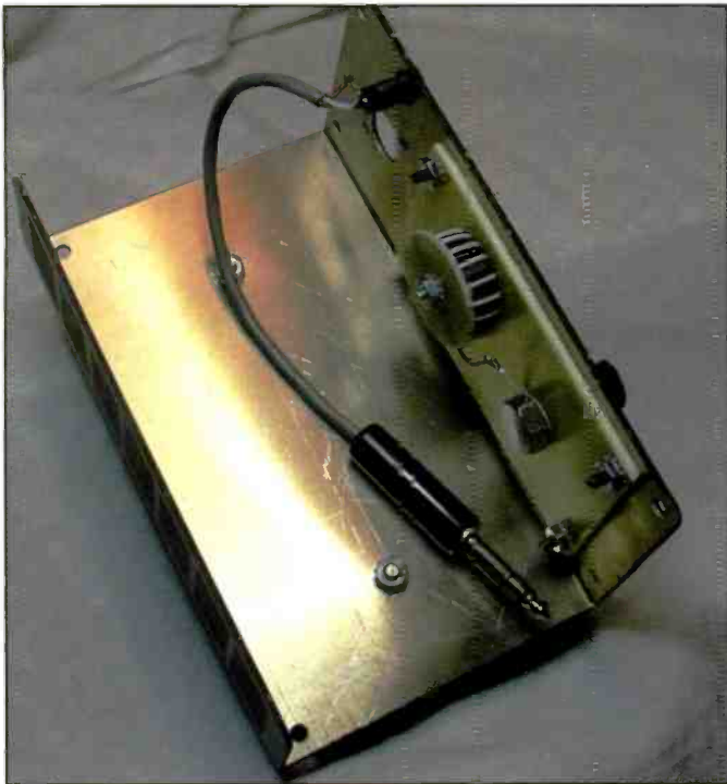
Photo I. Key jack wiring.
