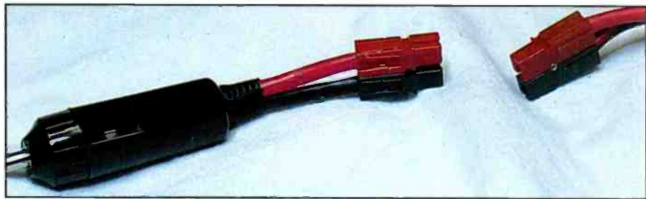
Photo D. Cut cable with PowerPoles.
